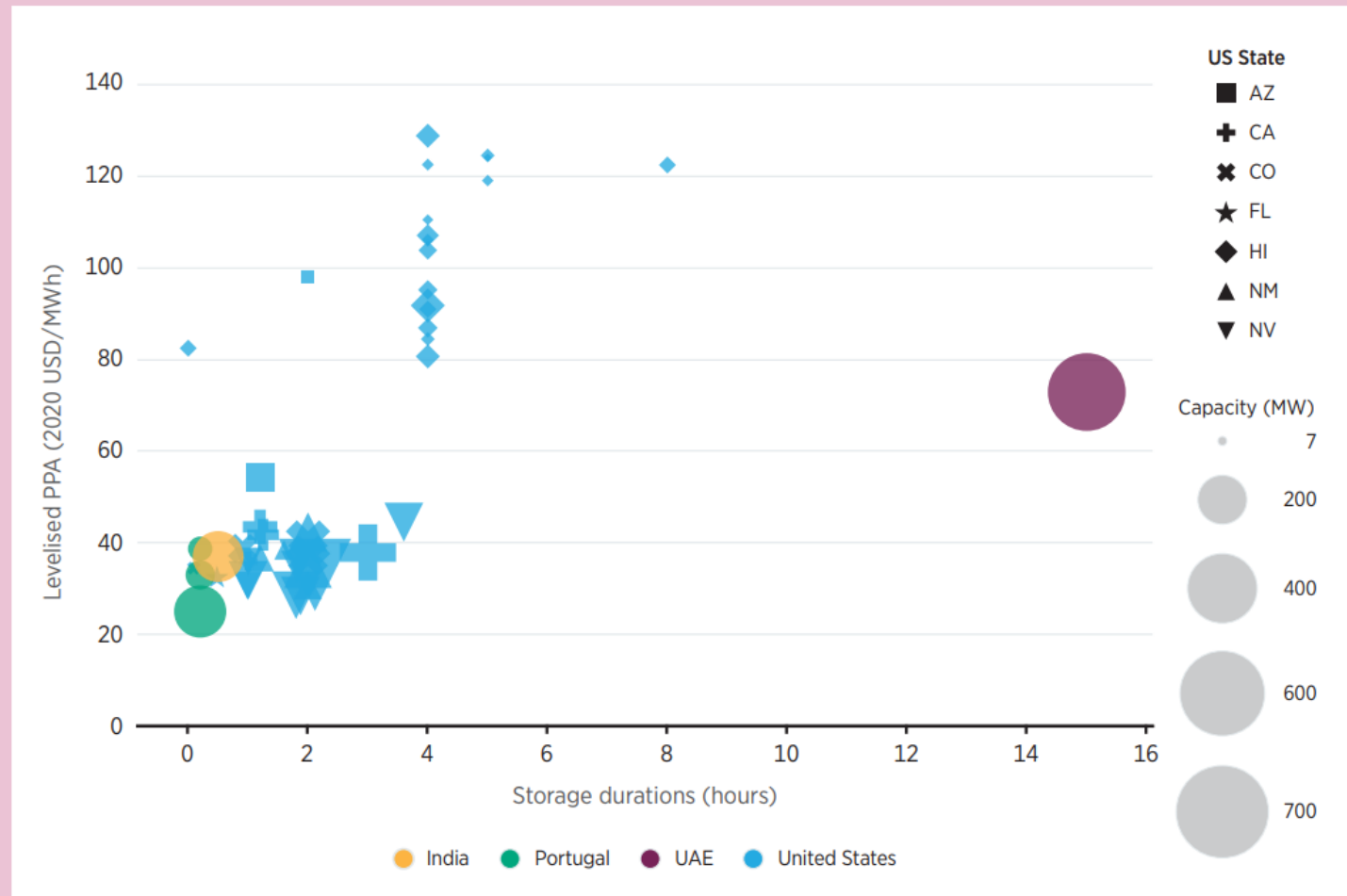
Figure B5.1 Results of recent auction and PPA results for utility scale solar PV and CSP
