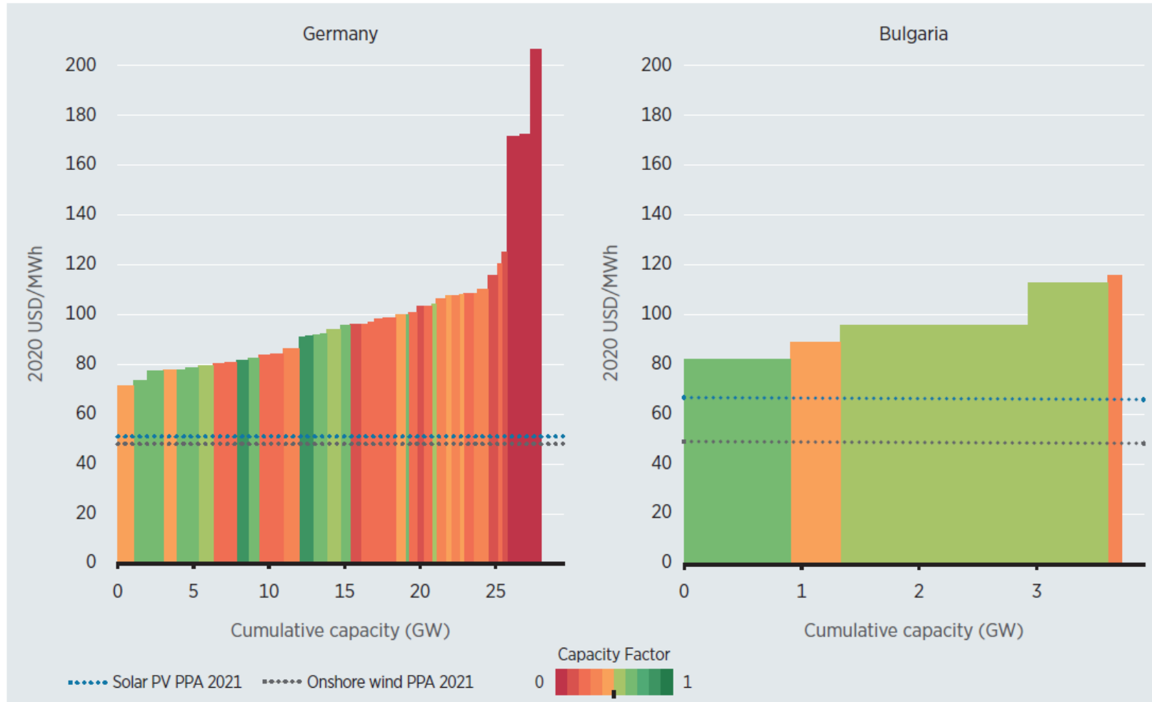
Figure 1.10 Operating costs only of existing coal-fired power plants in Bulgaria, Germany, India and the United States by installed capacity and capacity factor in 2020
