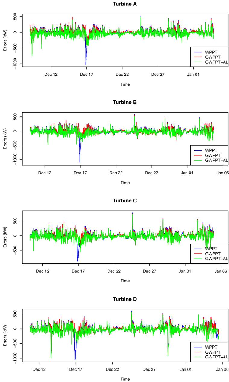
**Fig. 8.** Errors of WPPT, GWPPT and GWPPT-AL forecasts, time line (out-of-sample, 144 steps [24 hours] ahead). Turbines A to D, time frame October 31, 2010 to November 06, 2012.
