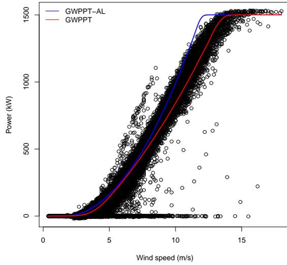
**Fig. 2.** GWPPT and GWPPT-AL in a power curve (in-sample). Turbine A, time frame October 31, 2010 to November 06, 2012.
