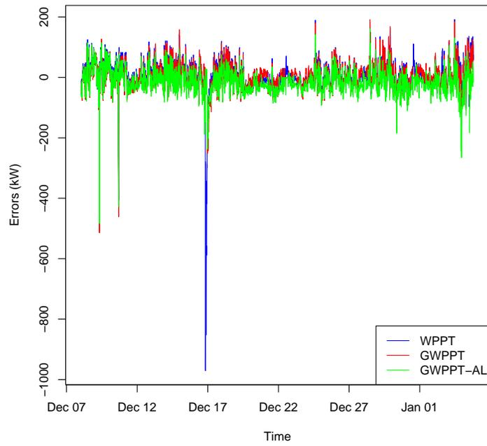
**Fig. 5.** Errors of WPPT, GWPPT and GWPPT-AL forecasts, time line (out-of-sample, 1 step [10 minutes] ahead). Turbine A, time frame October 31, 2010 to November 06, 2012.
