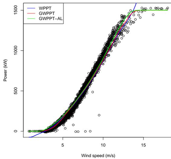
**Fig. 4.** WPPT, GWPPT and GWPPT-AL in a power curve (out-of-sample, 1 step [10 minutes] ahead). Turbine A, time frame December 08, 2011 to January 04, 2012.
