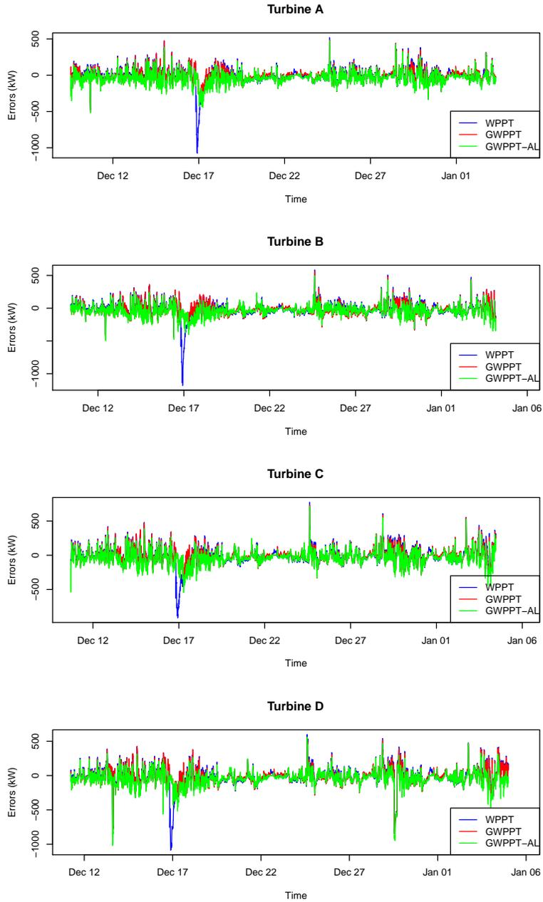
**Fig. 9.** Errors of WPPT, GWPPT and GWPPT-AL forecasts, time line (out-of-sample, 216 steps [36 hours] ahead). Turbines A to D, time frame October 31, 2010 to November 06, 2012.
