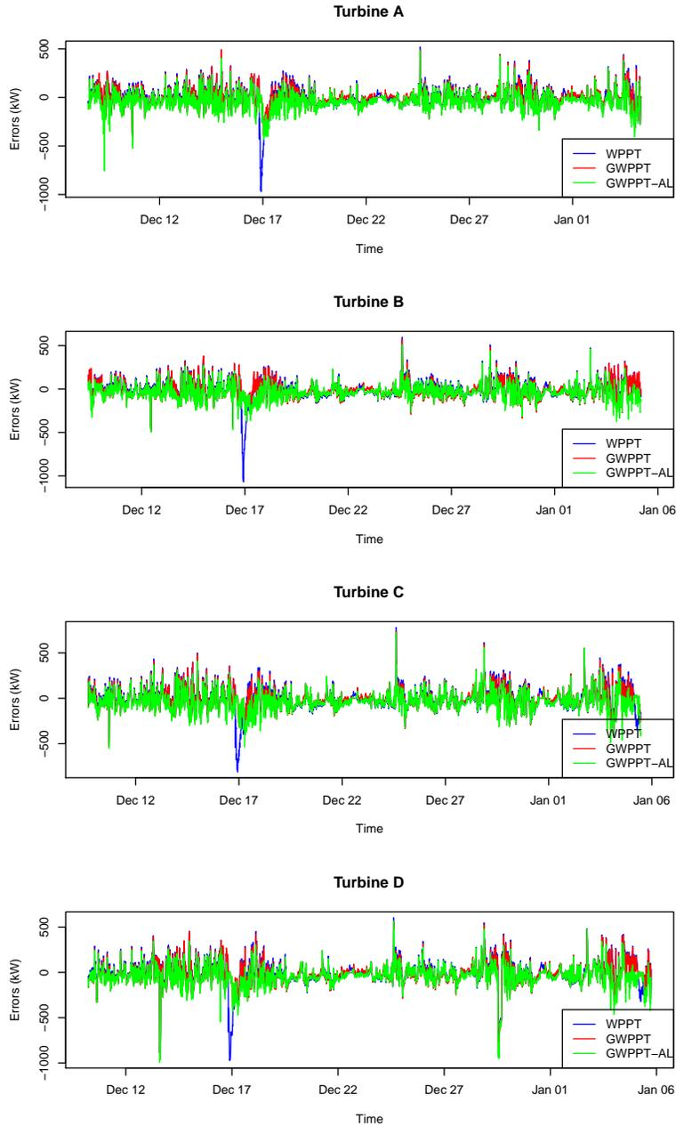
**Fig. 7.** Errors of WPPT, GWPPT and GWPPT-AL forecasts, time line (out-of-sample, 72 steps [12 hours] ahead). Turbines A to D, time frame October 31, 2010 to November 06, 2012.
