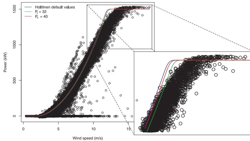
**Fig. 3.** Sensitivity analysis: Holttinen's default values,  $P_P = 40$  and  $P_I = 32$  in comparison. Turbine A, time frame October 31, 2010 to November 06, 2012.
