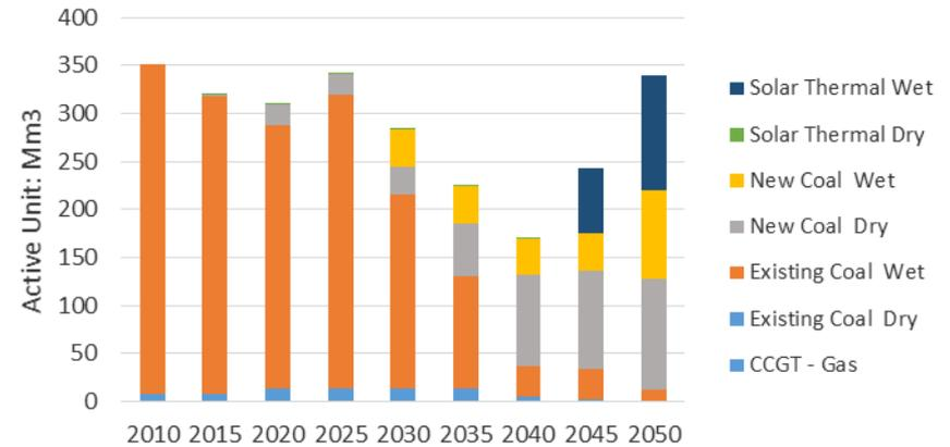
In the later planning periods wet-cooled solar thermal plants are preferred with ~4 GW of new wet-cooled coal due to a basic economic benefit of allocating available water to power generation.
