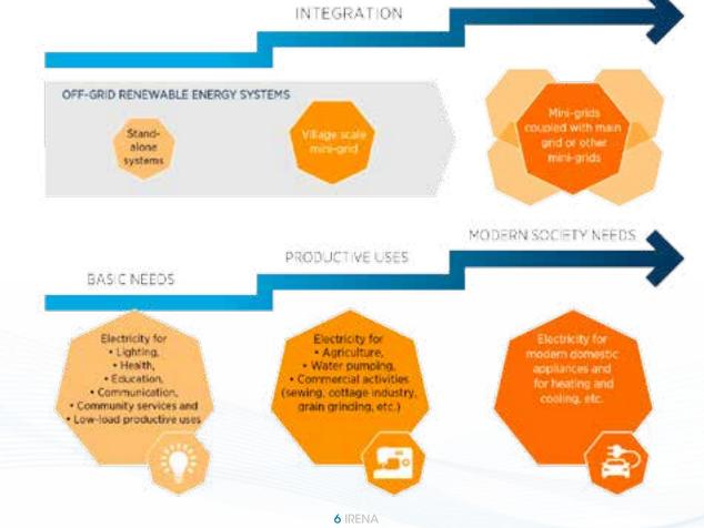
National energy access plans should therefore consider off-grid renewable energy options as part of a broader strategy towards universal access. By establishing a basic demand profile for an area, stand-alone systems can prepare the ground and build the economic foundation for larger systems, including mini-grids. Mini-grids may be further integrated into regional mini-grids or the main grid where technically feasible.
