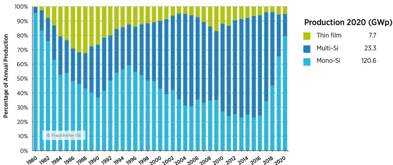
**Notes:** Mono-Si = monocrystalline silicon; Multi-Si = multi-crystalline silicon.
