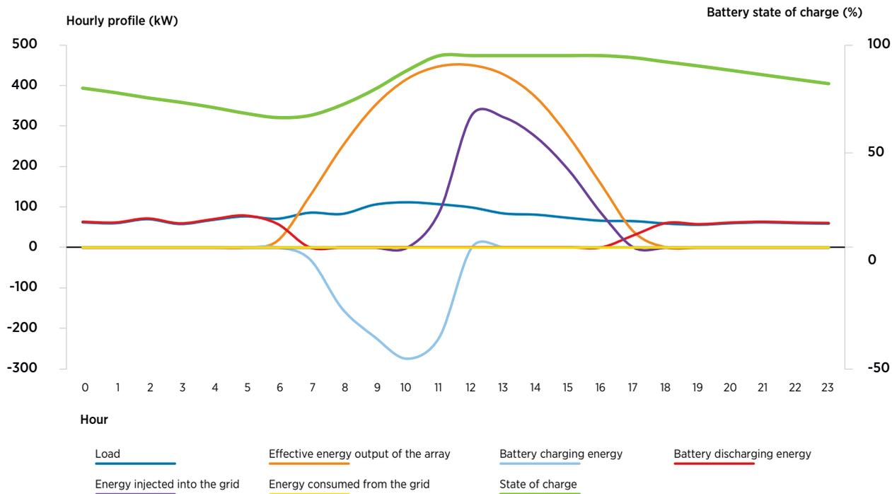
**Figure 58:** Hourly profiles on 3 October for configuration 7 of the solar PV system
