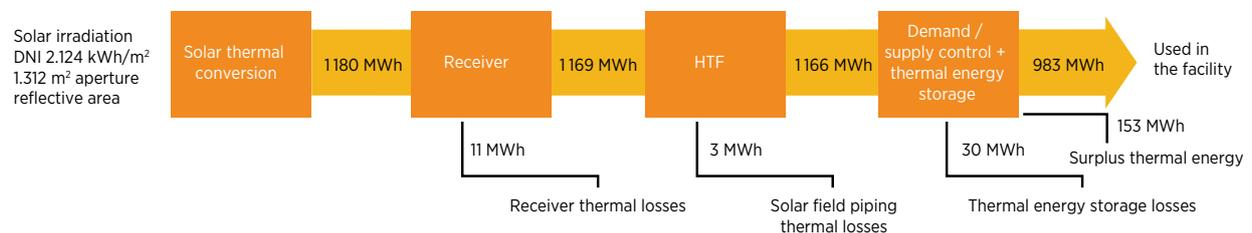
**Note:** DNI = direct normal irradiance; HTF = heat transfer fluid.
