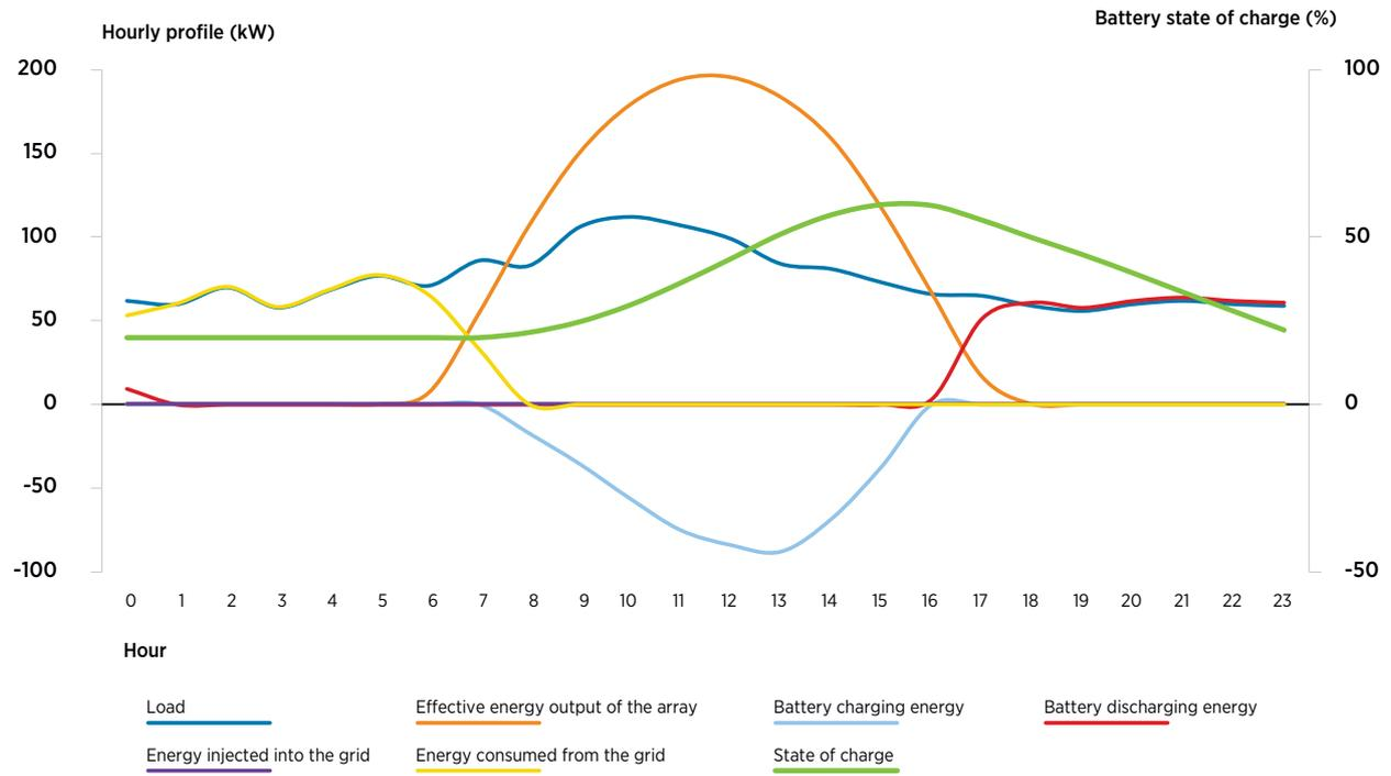
**Figure 56:** Hourly profiles on 3 October for configuration 3 of the solar PV system
