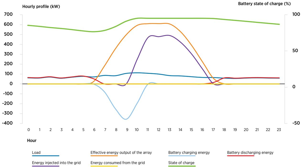
**Figure 60:** Hourly profiles on 3 October for configuration 10 of the solar PV system
