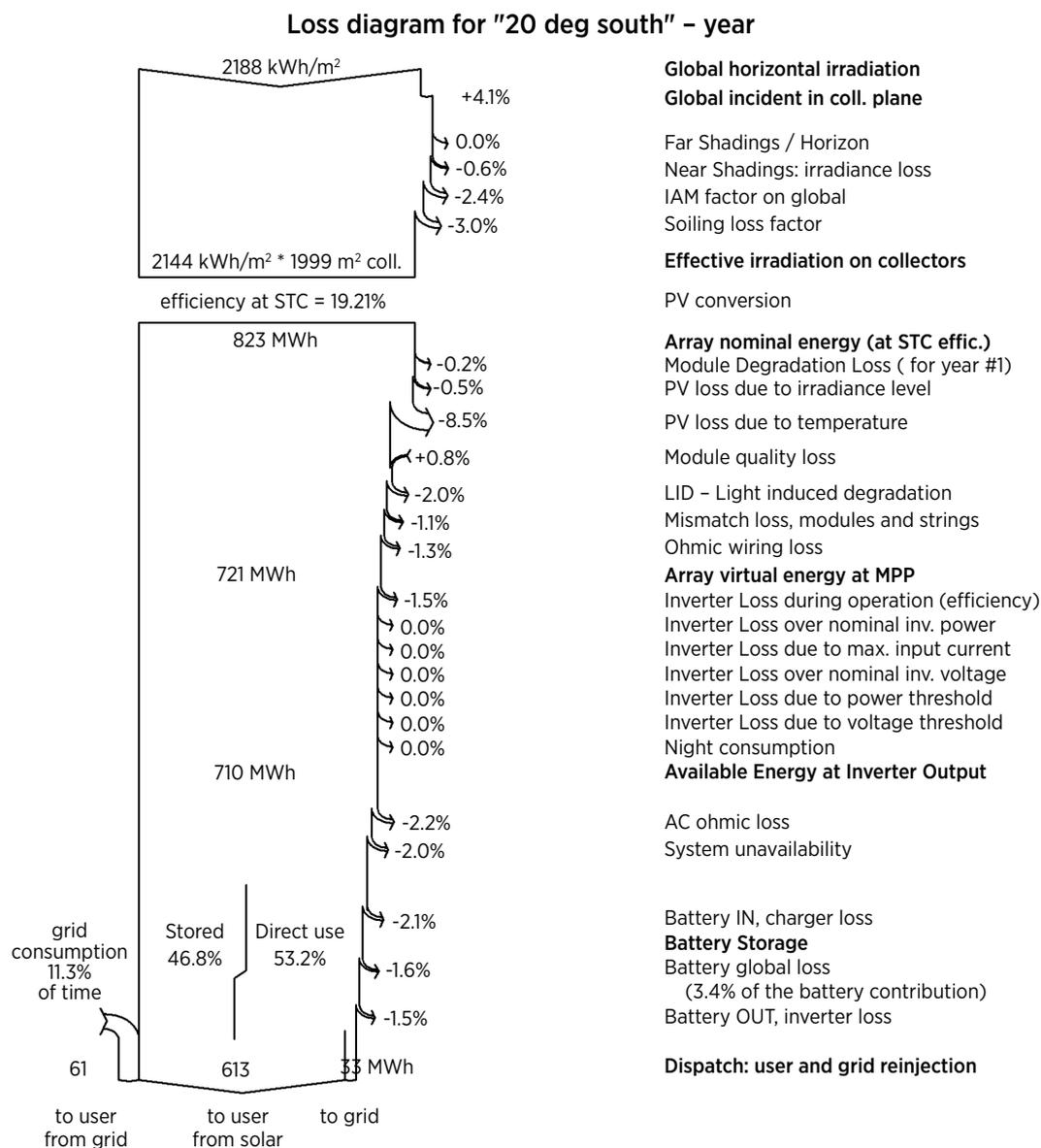
**Notes:** kWh = kilowatt hours; m<sup>2</sup> = square metre; STC = standard test conditions; MWh = megawatt hours; AC = alternating current; IAM = incidence angle modifier; MPP = maximum power point; coll. Plane = collector plane.
