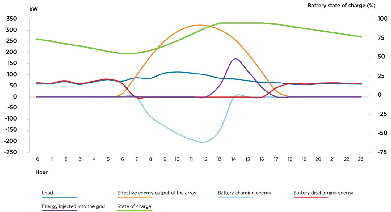
**Figure 27:** Hourly profiles on 3 October for configuration 5 of the solar PV system
