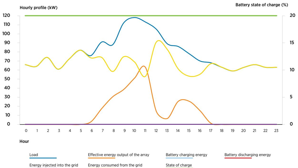
**Figure 55:** Hourly profiles on 13 March for configuration 3 of the solar PV system
