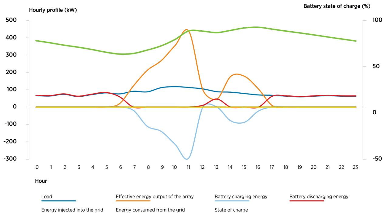
**Figure 59:** Hourly profiles on 13 March for configuration 10 of the solar PV system
