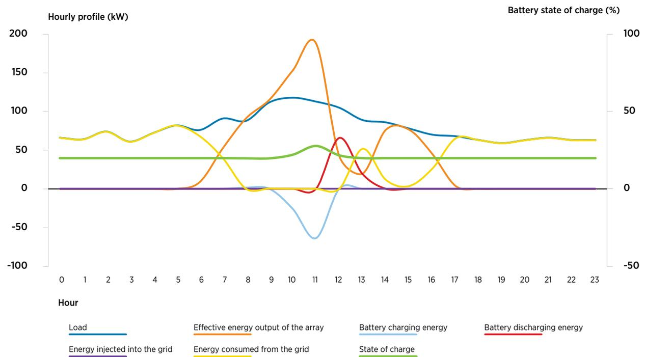
**Figure 57:** Hourly profiles on 13 March for configuration 7 of the solar PV system
