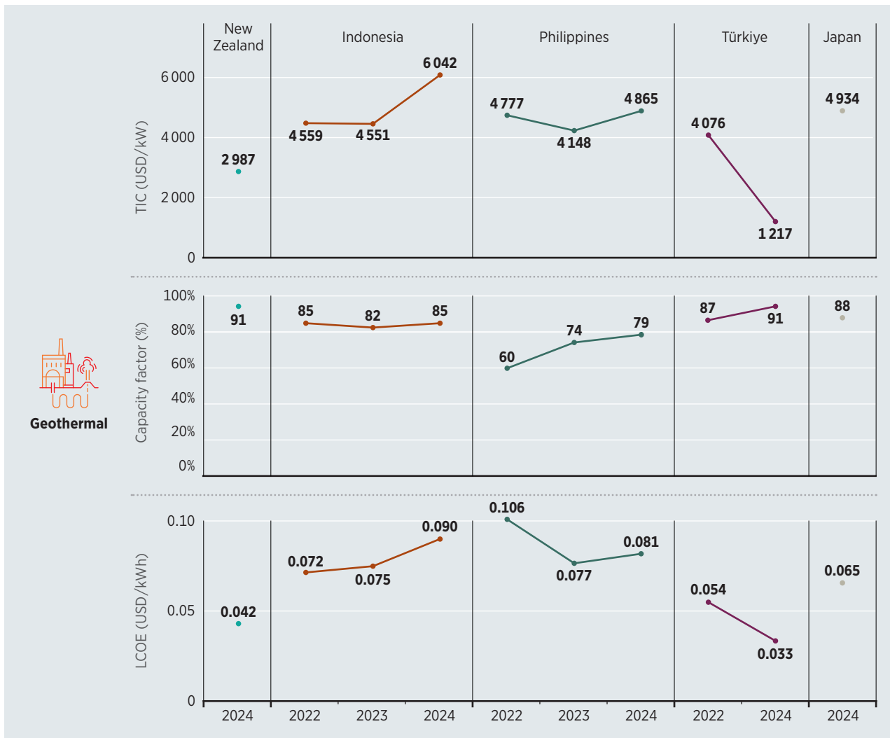
Figure 1.17 Geothermal power cost and performance trajectories in selected countries, 2022-2024
