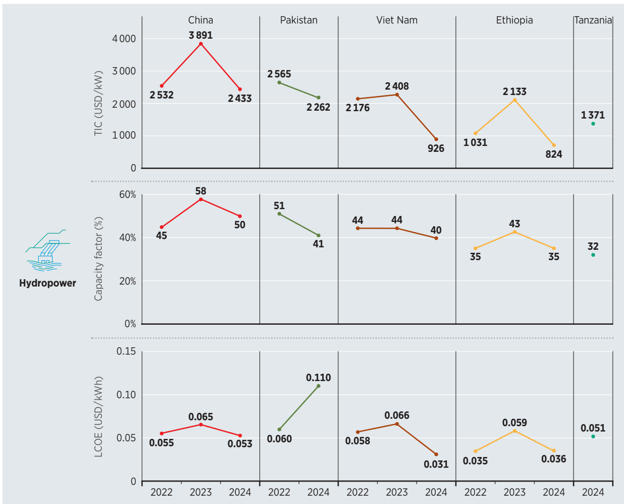
Figure 1.16 Hydropower cost and performance trajectories in selected countries, 2022-2024
