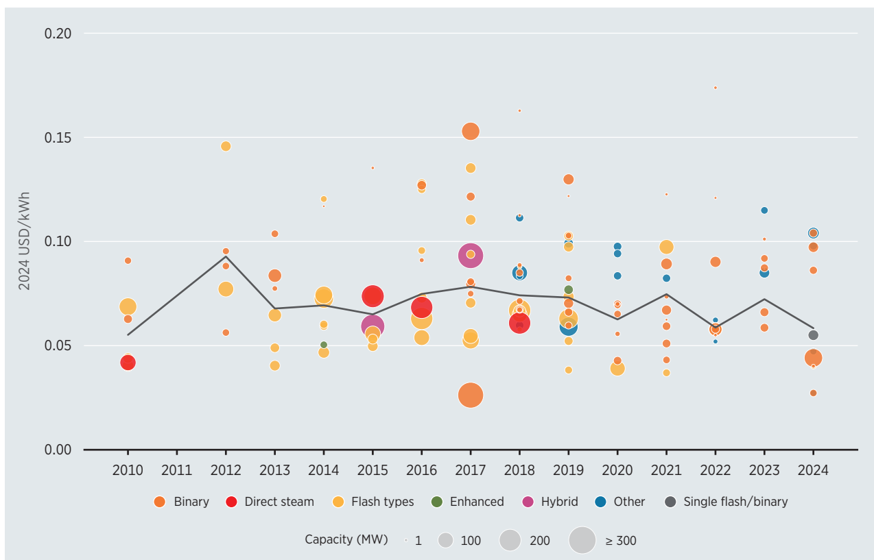
Figure 7.4 LCOE of geothermal power projects by technology and project size, 2010–2024
