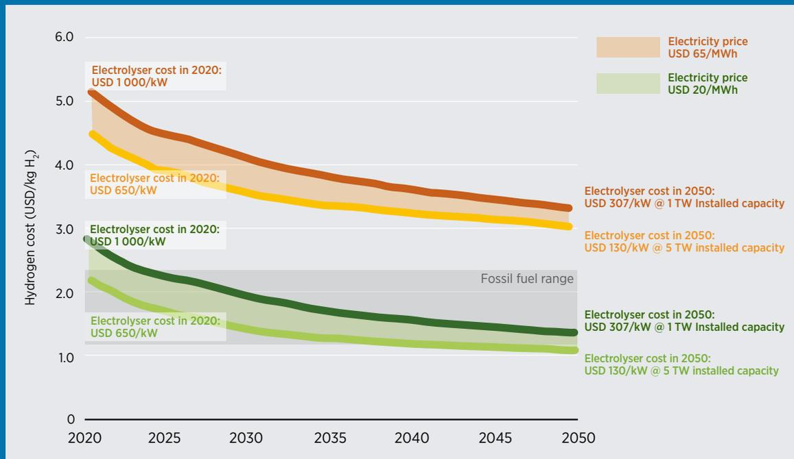
Note: Efficiency at nominal capacity is 65%, with a LHV of 51.2 kilowatt hour/kilogramme of hydrogen (kWh/kg H<sub>2</sub>) in 2020 and 76% (at an LHV of 43.8 kWh/kg H<sub>2</sub>) in 2050, a discount rate of 8% and a stack lifetime of 80 000 hours. The electrolyser investment cost for 2020 is USD 650-1000/kW. Electrolyser costs reach USD 130-307/kW as a result of 1-5 TW of capacity deployed by 2050.
