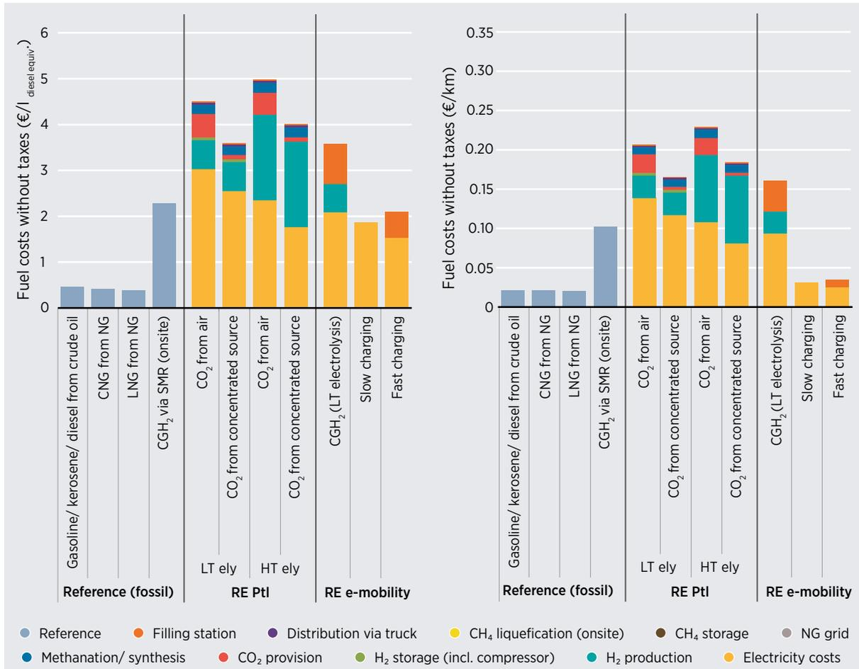
Notes: Left graph unit = EUR per litre of diesel equivalent; right graph unit = EUR per km; CGH<sub>2</sub> = compressed hydrogen; CNG = compressed natural gas; CH<sub>4</sub> = methane; H<sub>2</sub> = hydrogen; LNG = liquefied natural gas; LT = low temperature; HT = high temperature; NG = natural gas; SMR = steam methane reforming.
