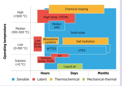
Notes: cPCM = composite phase-change material; PCM = phase-change material; WTTS = water thank thermal energy storage.
