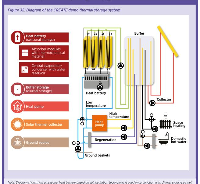
as heat pumps and solar thermal collectors.
