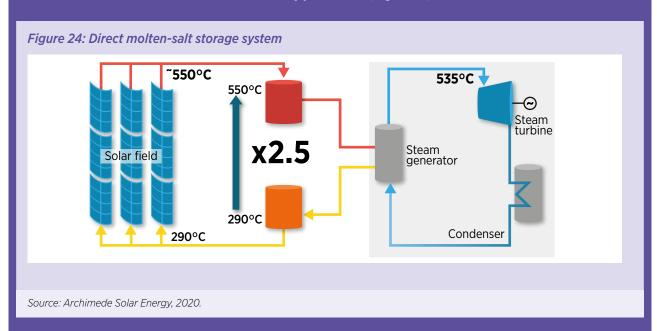
A two-tank molten-salt storage system is one of the most common configurations used (Figure 25). The molten salt is pumped between a cold and a hot storage tank for charging and discharging. Indirect systems use a heat exchanger with a heat transfer fluid cycle, whereas in direct systems the salt is used as both the storage medium and heat transfer fluid.
