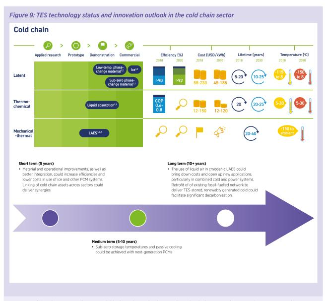
Note: Magnifying glass means value not available due to low technology readiness level; Flag means demonstration stage; Megaphone means commercial stage; (1) For the storage of cold; (2) For refrigerated transportation; (3) For the production of cold.
