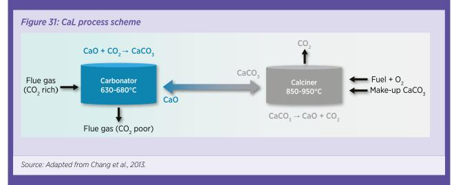
The advantage of the CaL system is that all materials involved are very low cost, and an extremely high energy density of 3.2 gigajoule per m3 can be obtained (Chang et al., 2013). However, the working temperatures involved are very high (> 600°C).
