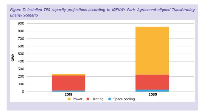
Note: Heating projections are not in the scope of this analysis due to a lack of data on aquifers and small-scale distributed TES (e.g. residential water tanks). Nonetheless, growth in the installed capacity of these technologies is expected given their versatile use from short to seasonal scale.
