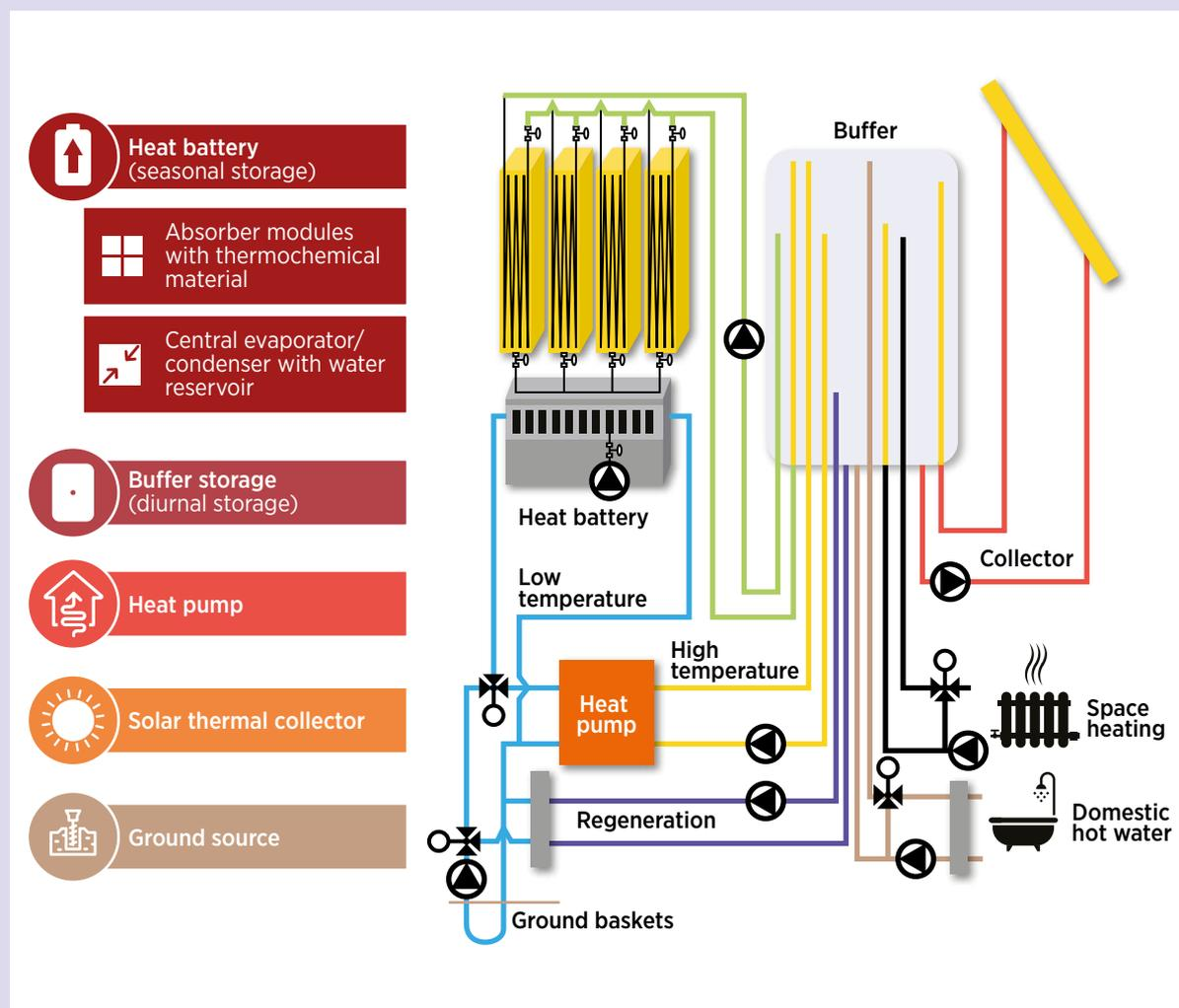
Note: Diagram shows how a seasonal heat battery based on salt hydration technology is used in conjunction with diurnal storage as well as heat pumps and solar thermal collectors.
