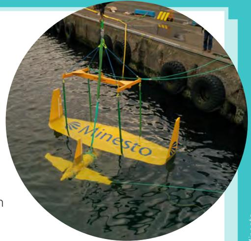
*Figure 19: Minesto's tidal kite device*
