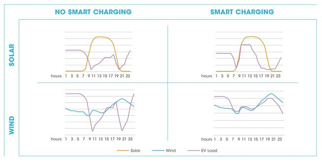
Figure 3: Smart charging for solar and wind generation profiles
