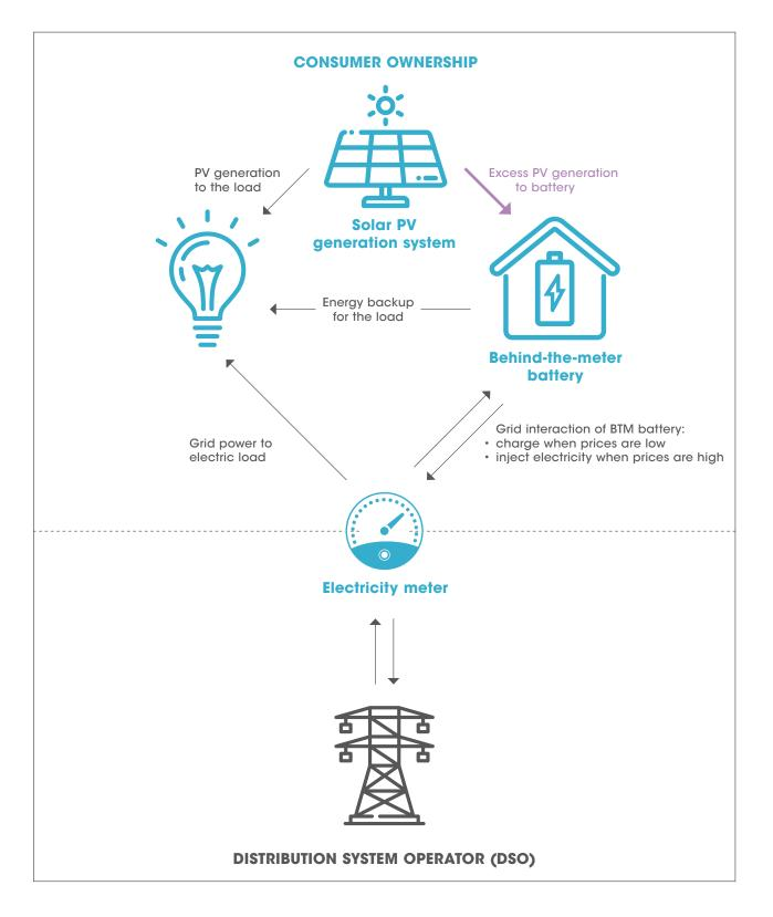
Figure 1: Grid-connected BTM energy storage configuration
