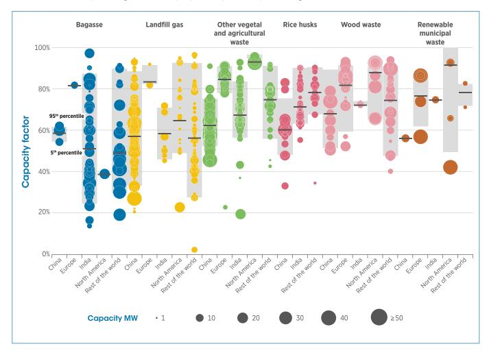
Capacity factors for individual projects typically span the 25-90% range, with weighted averages by technology and region ranging from 39% to 93%. Capacity factors for bagasse are lower than for other feedstocks, reflecting the seasonal availability of feedstock supplies.
