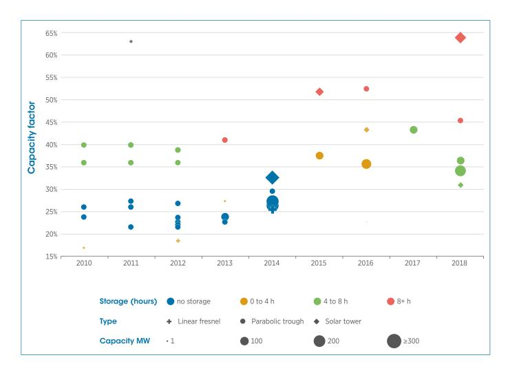
Capacity factors for new CSP plants increased between 2012 and 2018, with storage capacities growing and projects increasingly being developed in areas with better solar resources. New CSP projects commissioned in 2018 have estimated capacity factors ranging from 31% to 64%.
