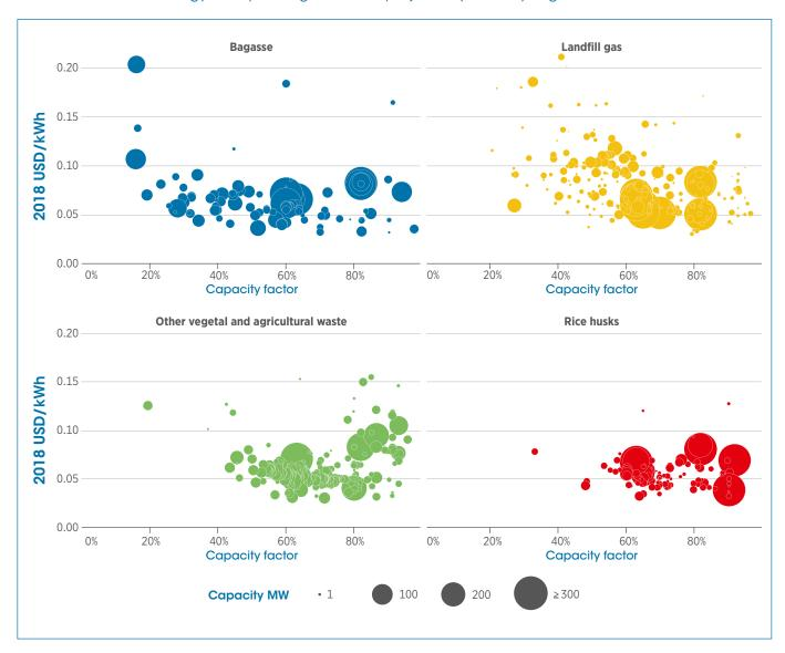
Bagasse plant LCOEs typically fall between USD 0.03/kWh and USD 0.08/kWh, with capacity factors ranging from 40% to 90%. LCOEs for landfill gas projects have lower LCOEs at higher capacity factors, while some larger projects utilising "other vegetal and agricultural waste" (with higher feedstock costs) tend to have higher LCOEs. Bioenergy projects using rice husks as feedstocks tend to have LCOEs between USD 0.03 and USD 0.07/kWh, for capacity factors between 50% and 90%.
