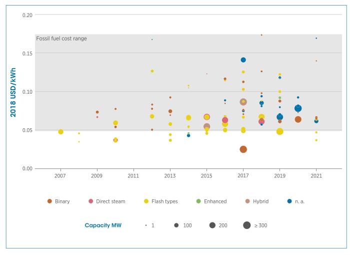
Most geothermal power projects have LCOEs between USD 0.05 and USD 0.08/kWh, which is at the lower end of the fossil-fuel cost range. Between 2013 and 2015, the weighted-average LCOE was around USD 0.06/kWh, rising to around USD 0.07/kWh during 2016-2018.
