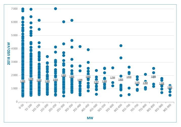
**Note:** For each capacity range presented the horizontal line represents the weighted average total installed cost for projects in that capacity range.
