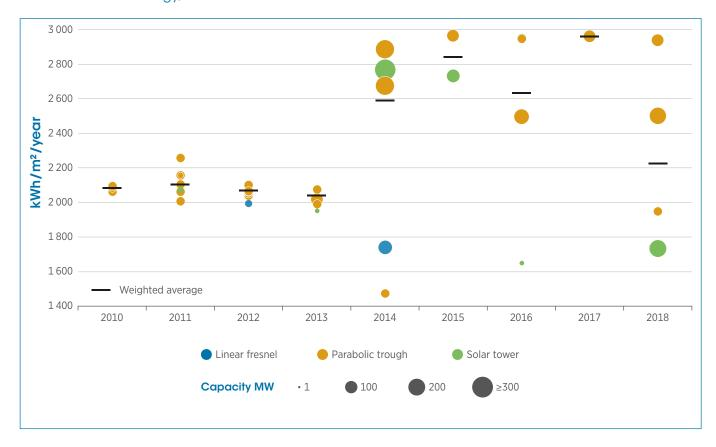
One driver of higher capacity factors in recent years is deployment in areas with higher direct normal irradiance (DNI). CSP projects commissioned in Spain in 2010–2013 were typically sited in areas with DNI in the 2000–2200 kWh/m2/year range, while sites with DNI of 2500–3000 kWh/m2/year became the norm in 2014–2018.
