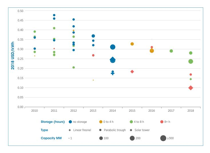
The combination of increasing capacity factors and falling installed costs has seen the LCOE of new CSP projects fall from between USD 0.27-0.48/kWh in 2010 and 2011 to USD 0.10-0.28/kWh in 2018. No projects have been built without storage since 2014, given that including storage minimises LCOE.
