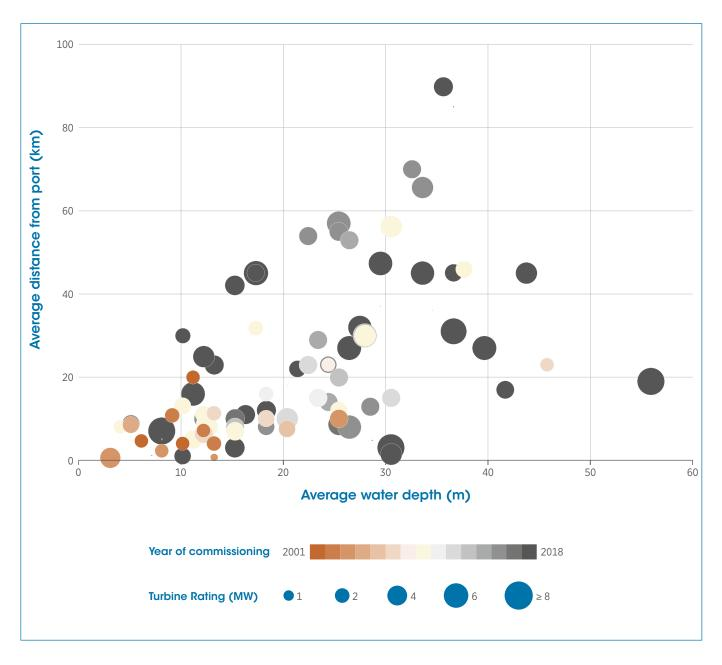
New offshore wind projects have moved to deeper waters and further offshore. Projects in recent years have typically been built at water depths between 10 m and 55 m and up to 90 km offshore, compared to around 10 m water-depth in 2001-2006, when distances to port rarely exceeded 20 km.
