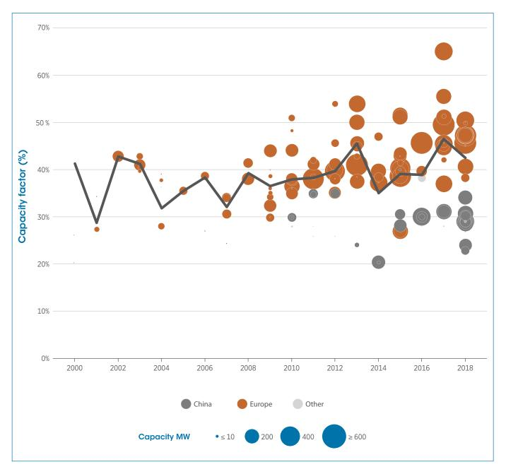
Capacity factors are higher in Europe (38% to 50% in 2018) than in China (23 to 34%), reflecting the relatively poorer wind resource and smaller turbines for near-shore Chinese projects. A clear trend to higher capacity factors for new offshore European wind farms can be seen since 2008, with average capacity factors rising from an average of around 35% to around 50% in 2017 and 2018.
