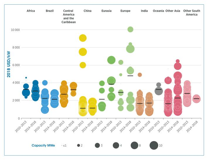
Note: Small hydropower projects in this figure are all those with capacity less than or equal to 10 MW.
