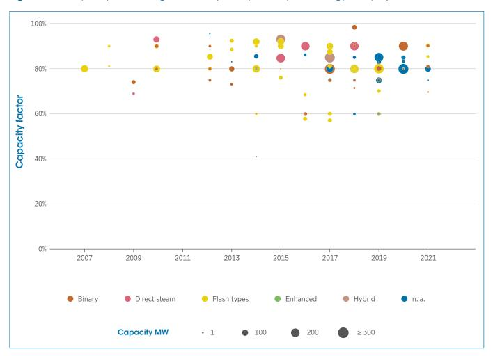
Capacity factors for geothermal plants are typically expected to be in the range of 80-90%, but lifetime capacity factors will depend heavily on well performance and ongoing investment to maintain production wells.
