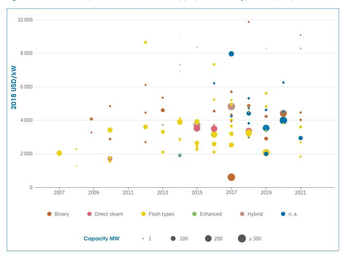
The market for geothermal power is relatively thin, leading to significant year-on-year variations in installed costs. Total installed costs for geothermal plants are typically between USD 2000 and USD 5000/kW. On average, the costs for "binary" geothermal plants are higher than those for "flash" types that exploit higher-temperature resources.
