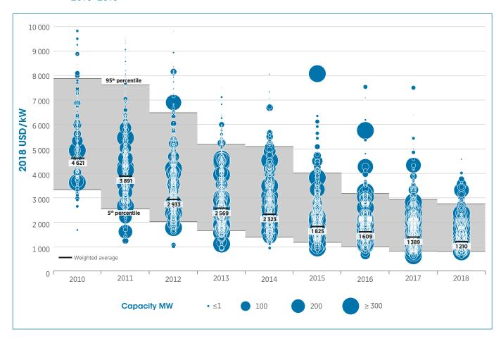
The global weighted-average total installed cost of utility-scale solar PV has fallen by 74% between 2010 and 2018. Installed costs have also converged closer to the average, with the 5th and 95th percentile range dropping from the USD 3300-7900/kW range in 2010 to USD 800-2700/kW in 2018. Utility-scale solar PV project investment costs have fallen from USD 4621/kW in 2010 to USD 1210/kW in 2018.
