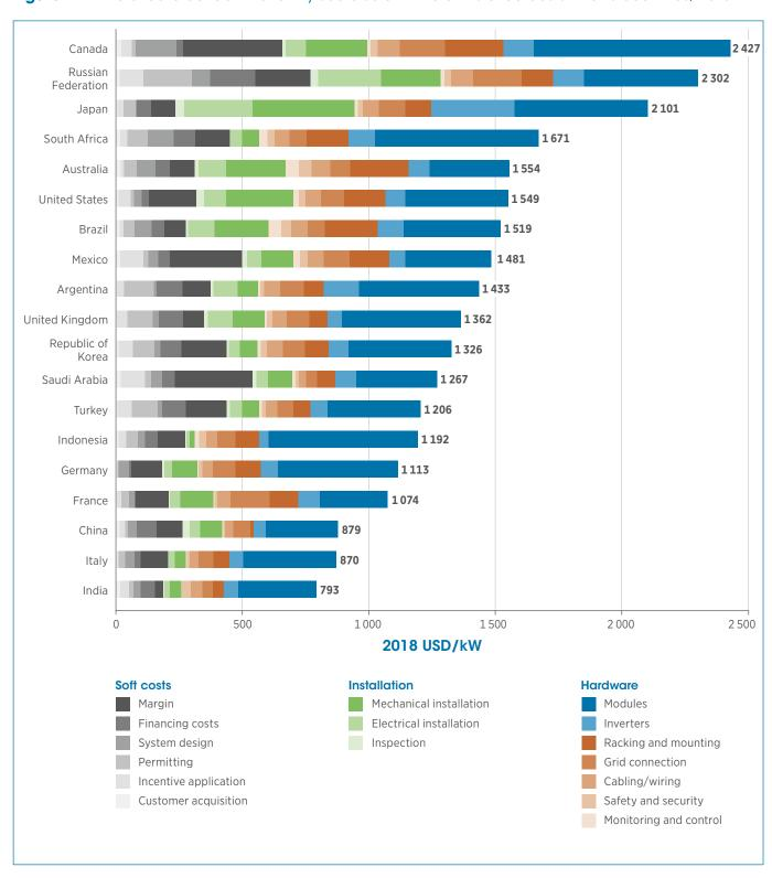
The country average for the total installed costs of utility scale solar PV in G20 countries ranged from a low of USD 793/kW in India to a high of USD 2427/kW in Canada in 2018. The lowest cost average was three times less than the highest, despite the convergence of installed costs in major markets in the last three years.
