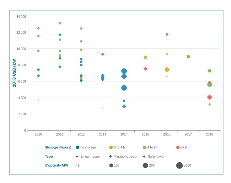
CSP investment costs have declined from the USD 6100-13100/kW range for up to eight hours storage between in 2010-2012, to USD 3200-7300/kW in 2018 for projects with higher storage capacities (4-8 hours or more). No Linear Fresnel designs have been installed since 2014.
