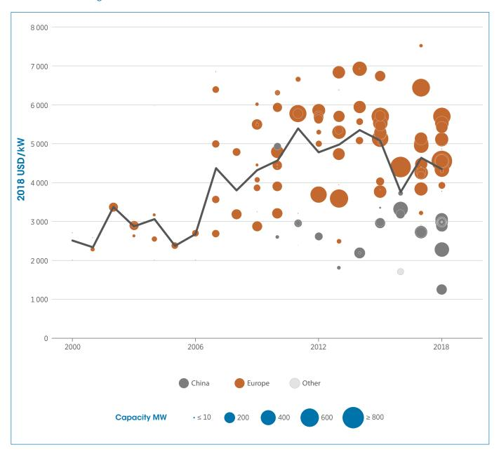
With the shift to deeper water and sites further from ports, the total installed costs of offshore wind farms rose, from an average of around USD 2500/kW in 2000 to around USD 5400/kW by 2011–2014, before falling to around USD 4350/kW in 2018. Total costs are higher in Europe than in China, reflecting the fact that Chinese deployment to date remains in shallow waters, close to ports.
