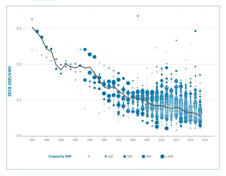
The global weighted-average LCOE for onshore wind fell by 82% between 1983 and 2018, over which time cumulative installed capacity grew to 540 GW.
