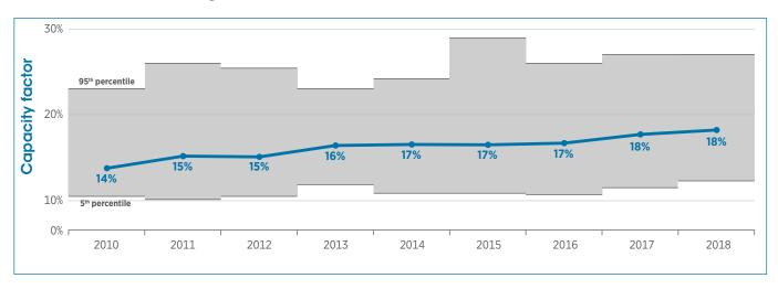
The global weighted-average capacity factor for new utility-scale solar PV, by year commissioned, has increased from 14% in 2010 to 18% in 2018 as the share of deployment in sunnier locations has risen.
