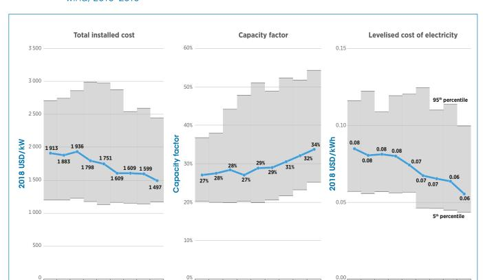
**Figure S.4** Global weighted average total installed costs, capacity factors and LCOE for onshore wind, 2010–2018
