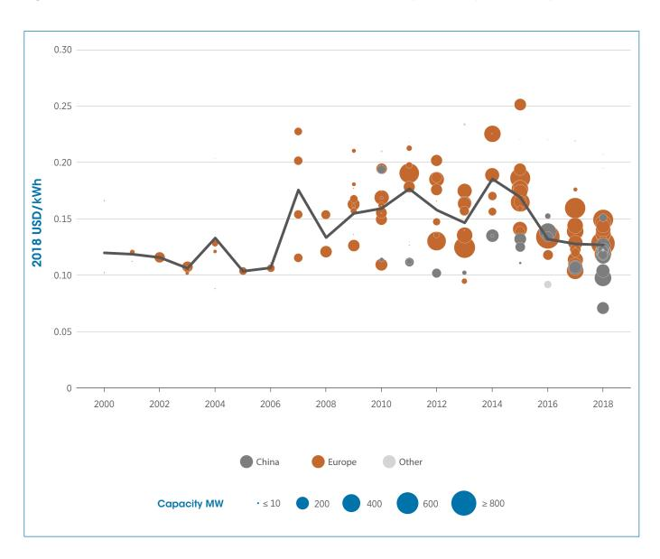
The global weighted-average LCOE of offshore wind projects commissioned in 2018 was USD 0.127/kWh. Like total installed costs, the average LCOE increased up to around 2011, before declining noticeably between 2016 and 2018. The weighted average LCOE was around USD 0.134/kWh in Europe in 2018. This was 28% higher than in China, where the value was around USD 0.105/kWh.
