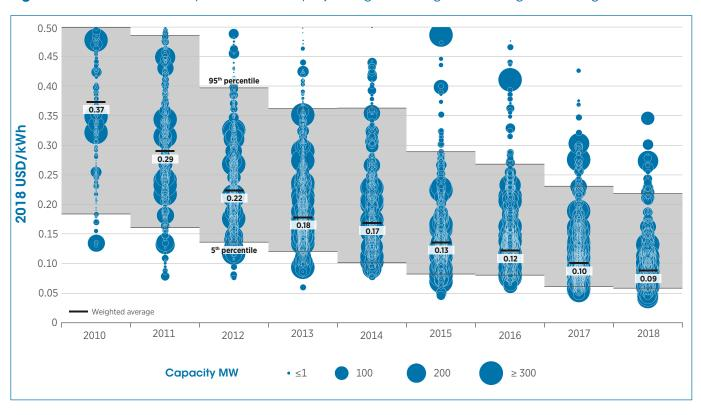
The global weighted-average LCOE of utility-scale solar PV declined by 77% between 2010 and 2018, from USD 0.371 to USD 0.085/kWh. Globally, although the range has narrowed, the 5th and 95th percentile for projects in 2018 ranged from USD 0.058 to USD 0.219/kWh.
