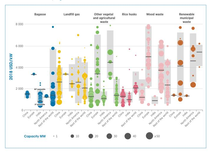
Differences in total installed costs for bioenergy are more significant between countries than feedstock types. Total installed costs vary significantly within countries or regions depending on the technology employed. Bioenergy projects using bagasse and rice husks as feedstocks tend to have lower installed costs than those using landfill gas, wood waste, other vegetal and agricultural waste and renewable municipal waste.
