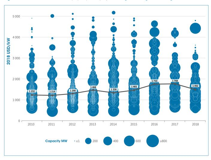
Installed costs for hydropower have increased from USD 1232/kW in 2010 to USD 1492/kW in 2018. Total installed costs span a wide range, reflecting the very site-specific nature of hydropower projects, but generally fall within the USD 1000-2500/kW range. In 2018, total installed costs fell from their recent highs in 2016 and 2017.
