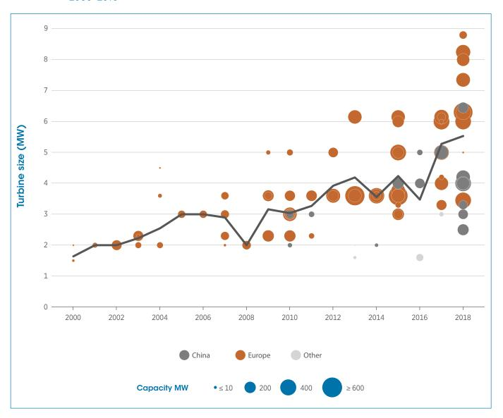
The average size of offshore wind turbines grew by a factor of 3.4 in less than two decades, from 1.6 MW in 2000 to 5.5 MW in 2018. Offshore wind farms commissioned in Europe in 2018 used turbines between 3.5 MW and 8.8 MW capacity.
