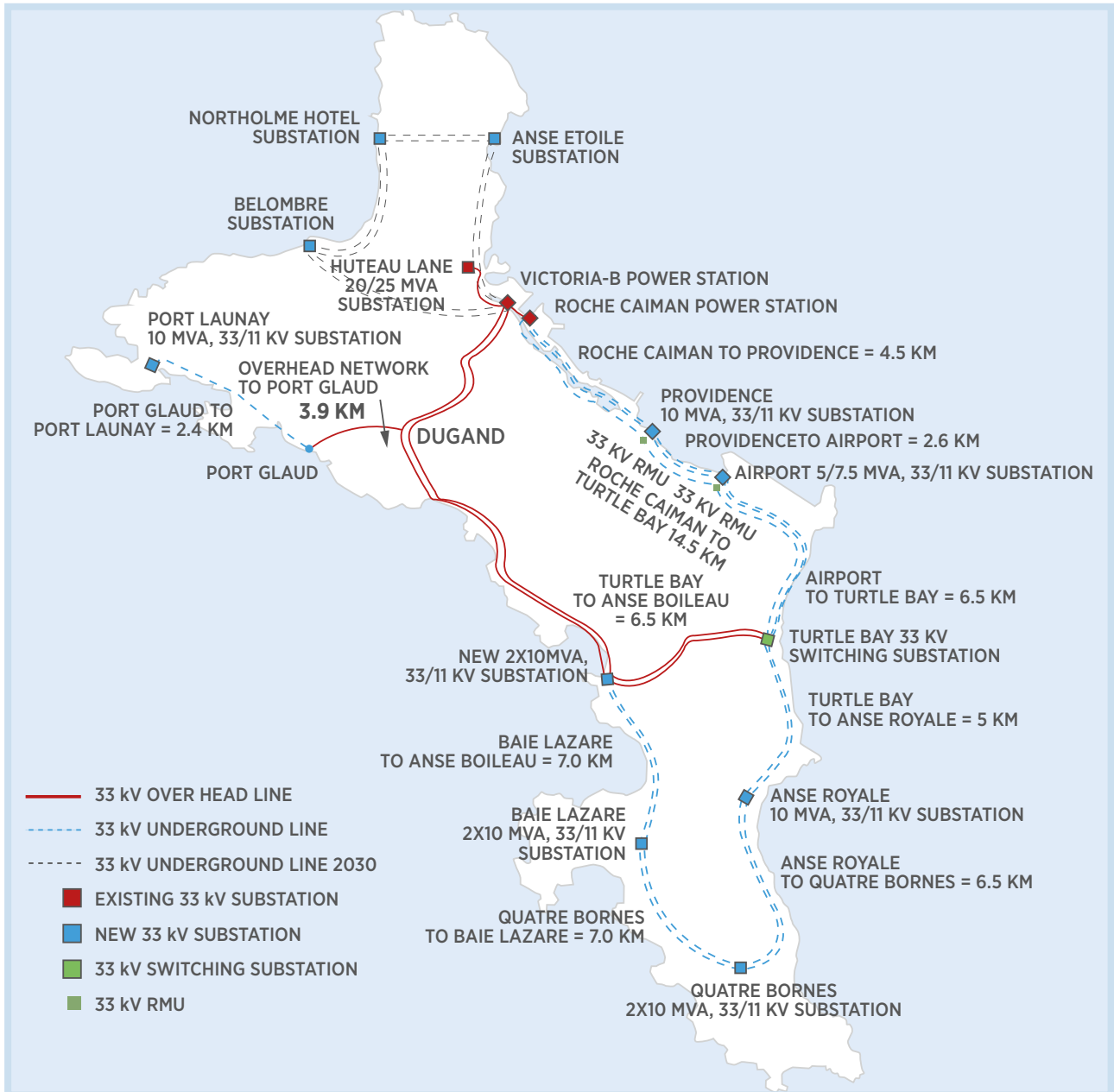
Figure 22: Electrical network of Mahé island
