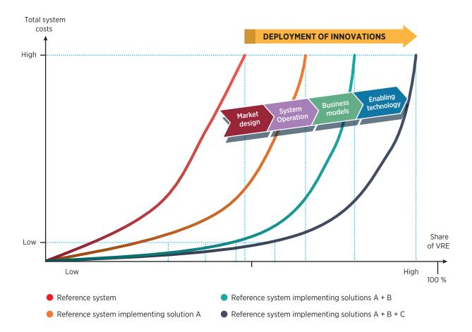
Figure S11 Concept of innovation reducing total system costs with high shares of VR
