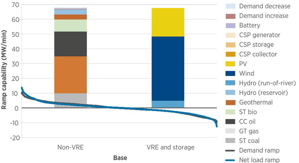
**Figure 13:** Net load ramp with upward and downward one-hour ramping capabilities
