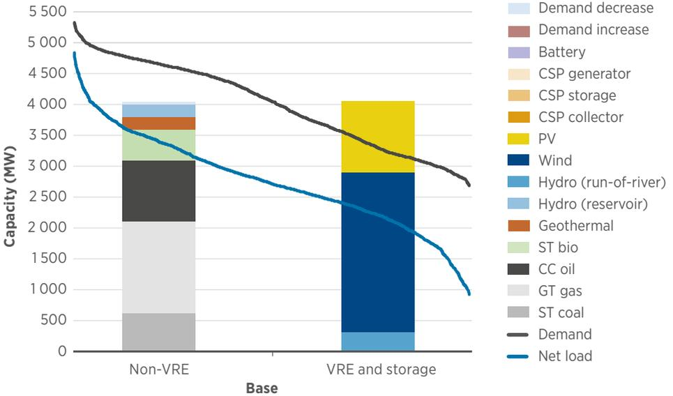
**Figure 12:** Ramp duration curve for demand and net load (change between two time periods) as well as upward ramping capabilities of units (leftmost column for conventional capacity and rightmost for VRE and storage)
