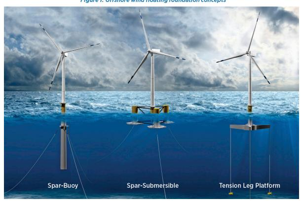
Figure 1: Offshore wind floating foundation concepts
