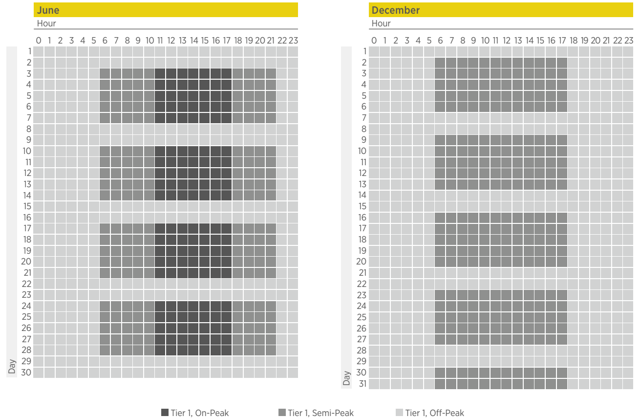
Figure 27: Quantity of hours in each TOU period for a weekday in June (summer season) and December (winter season) on SDG&E’s residential TOU schedule DR-SES
