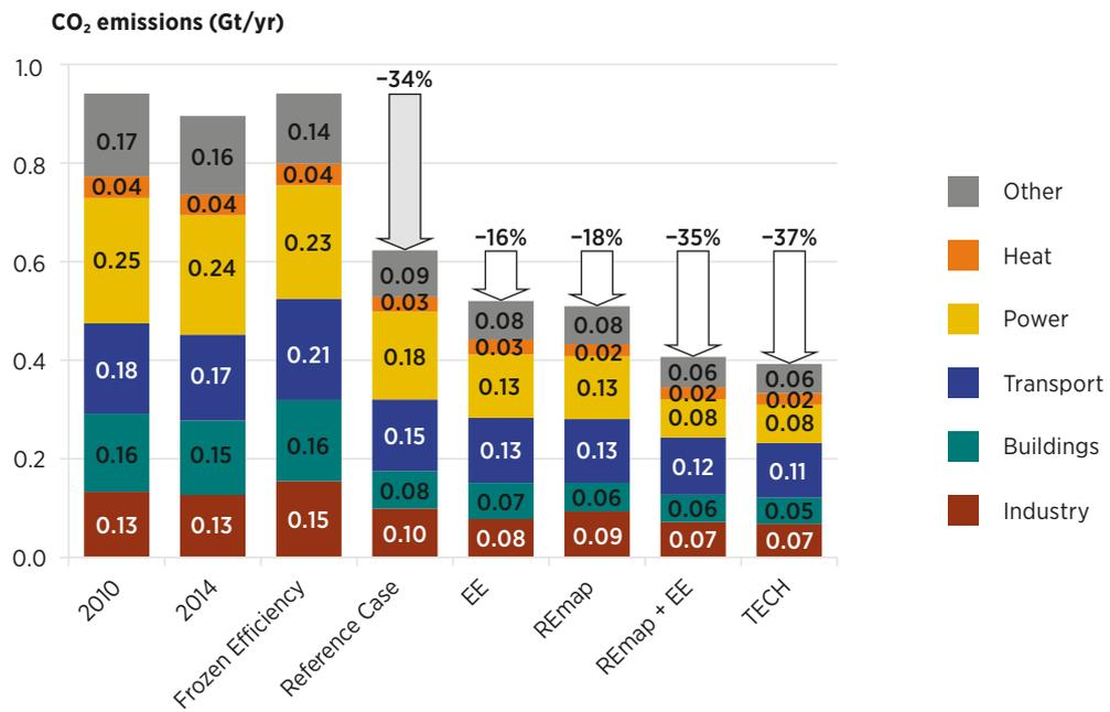
Note: For the REmap and EE cases, the relative decrease in CO<sub>2</sub> emissions is larger (17–18%) than the relative decrease in primary energy use (4–5%). This is mainly due to savings of coal-based electricity in the buildings and industrial sectors, as well as the shift from coal- to gas-fired power stations.
