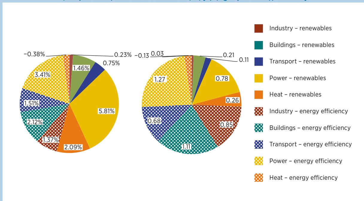
Note: The shift from fossil fuels to biomass results in a slightly lower generation efficiency for the heating sector, resulting in a TPES increase of 0.1 EJ/yr and renewable energy share decrease of 0.4%pt.
