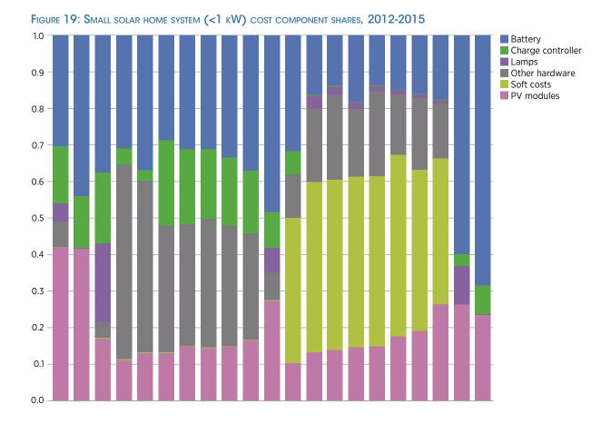
The battery makes up a significant cost component of these sub-1 kW SHS. The battery generally also has the shortest lifetime of any component, adding to its contribution to the lifetime cost of the product. While modules and LEDs will last 10-20 years or more, batteries often last 5 years or less and can require more maintenance. Battery replacement therefore will be an important component of the lifetime costs of SHS.
