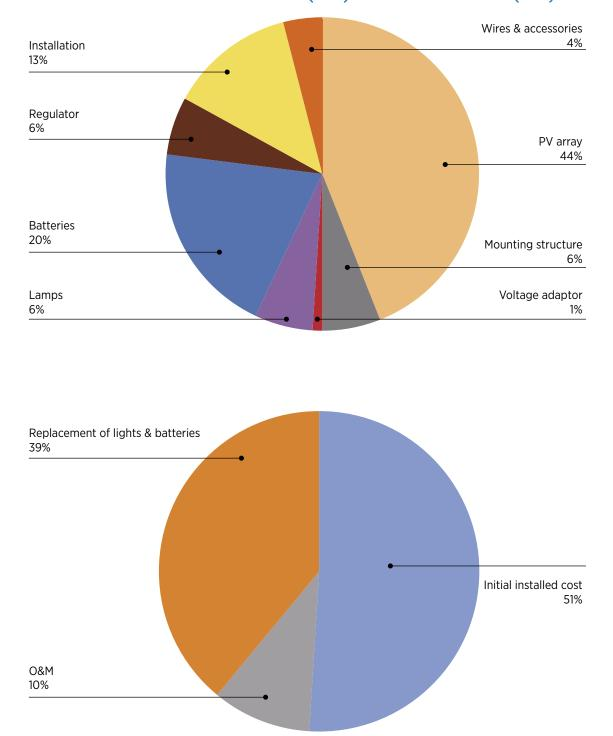
FIGURE 26: COST BREAKDOWN OF 100 WP SOLAR PV SYSTEM (ABOVE) AND ANNUALISED LIFE-CYCLE COST (BELOW) IN GHANA
