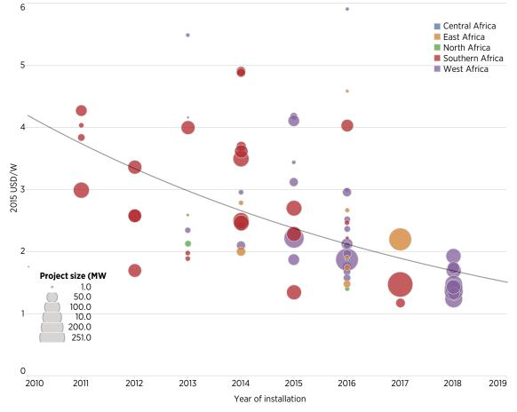
FIGURE 34: UTILITY-SCALE TOTAL INSTALLED COSTS BY PROJECT SIZE AND REGION FOR INSTALLATION, 2011-2018
