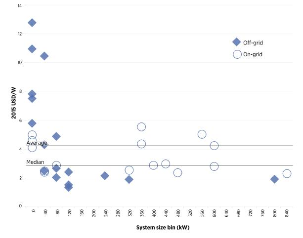
FIGURE 29: PV MINI-GRID SYSTEM COSTS BY SYSTEM SIZE IN AFRICA, 2011-2015
