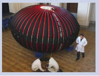
Figure 34: Small-scale demonstrator of underwater compressed-air energy storage system
