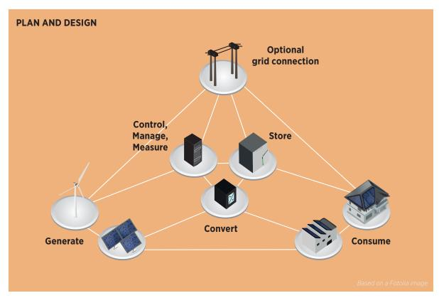
Mini-grids can be categorised based on their connection to the grid and the level of service provided. A renewable mini-grid can be interconnected to the main grid or independent from neighbouring grids, in which case it is considered autonomous. Renewable mini-grids can provide different levels of service, from basic services such as only lighting to higher levels of service, such as satisfying commercial energy demand. Table S1 provides an overview of these categories.
