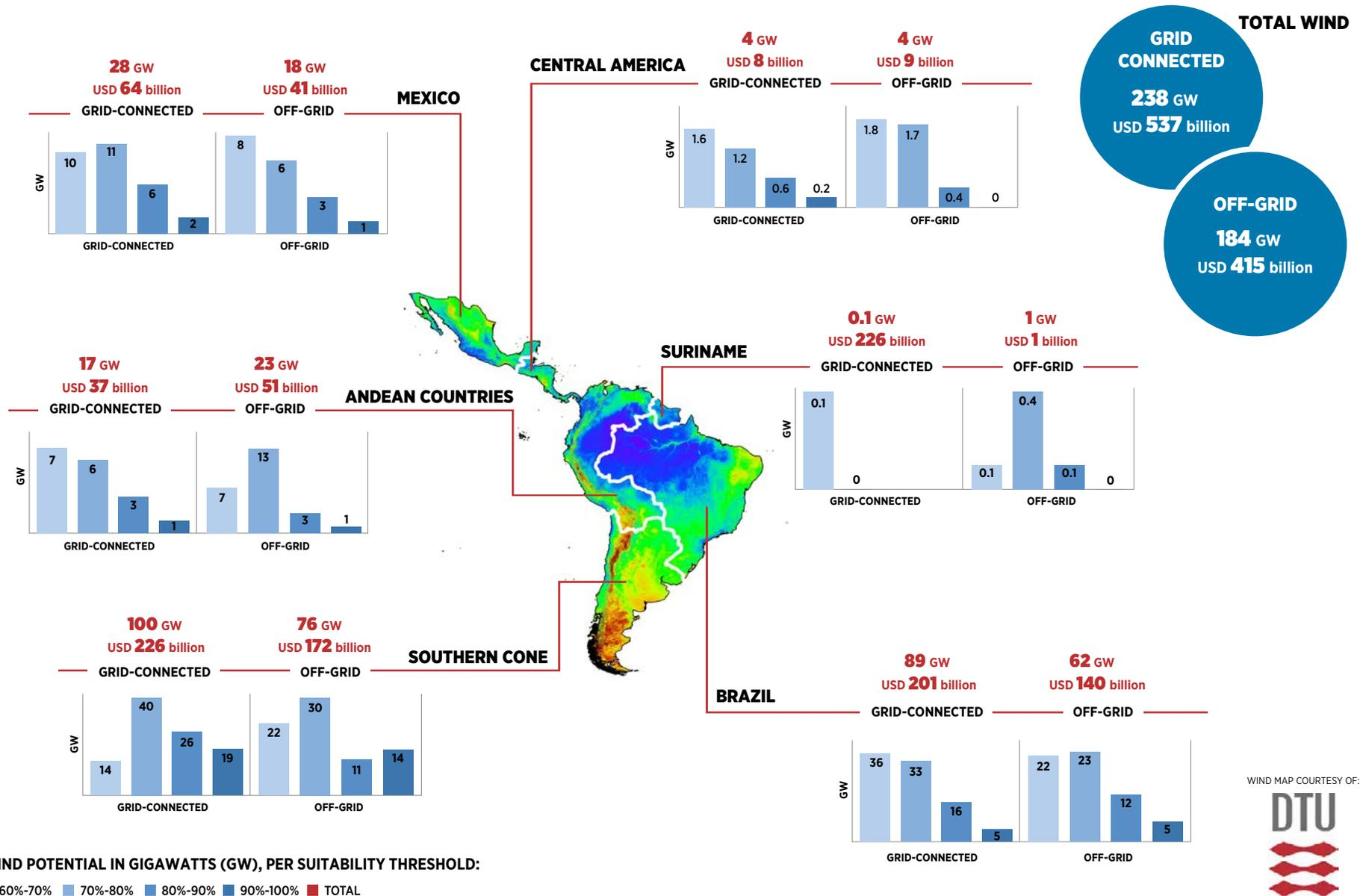
Figure 4: Wind energy - Grid-connected and utility-scale off-grid technical potential estimates for Latin American by region, expressed in GW and USD. The suitability threshold is 60% and the output is indicated for a grid distance of 75 km.
