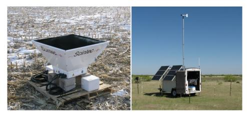
**Figure 8-2** *Left*: Scintec SFAS sodar unit. *Right*: Atmospheric Research & Technology VT-1 sodar unit enclosed within a trailer. (Source: AWS Truepower)
