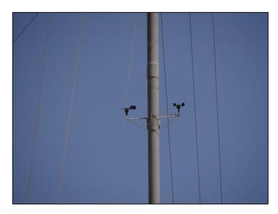
**Figure 7-4.** A poor sensor configuration. The anemometer booms are too short compared to the tower width, and likely would result in a large influence of the tower on the anemometer readings. (Source: AWS Truepower)
