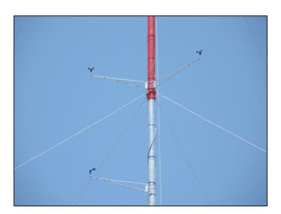
**Figure 7-3.** A good sensor configuration. The anemometer booms are long compared to the tower width, and the second anemometer is mounted at the recommended angle from the first. The vane is a good distance below. (Source: AWS Truepower)
