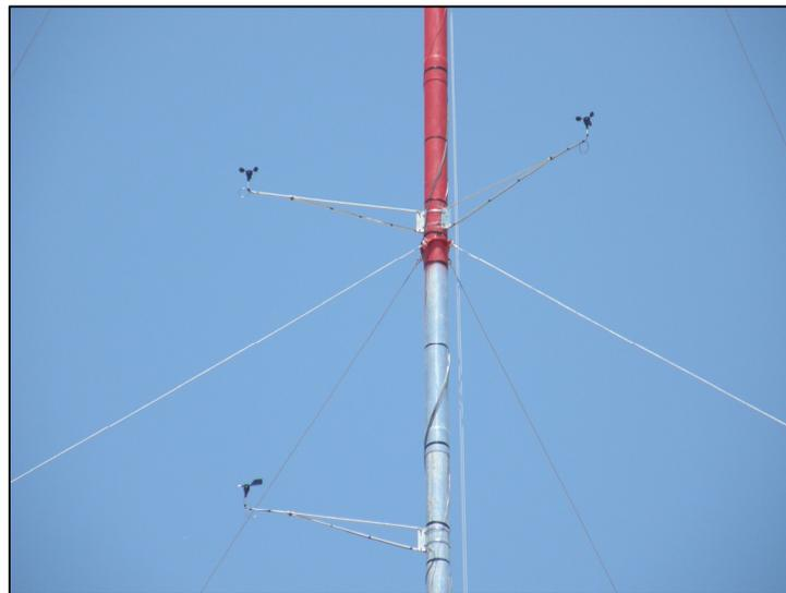
**Figure 7-3.** A good sensor configuration. The anemometer booms are long compared to the tower width, and the second anemometer is mounted at the recommended angle from the first. The vane is a good distance below. (Source: AWS Truepower)
