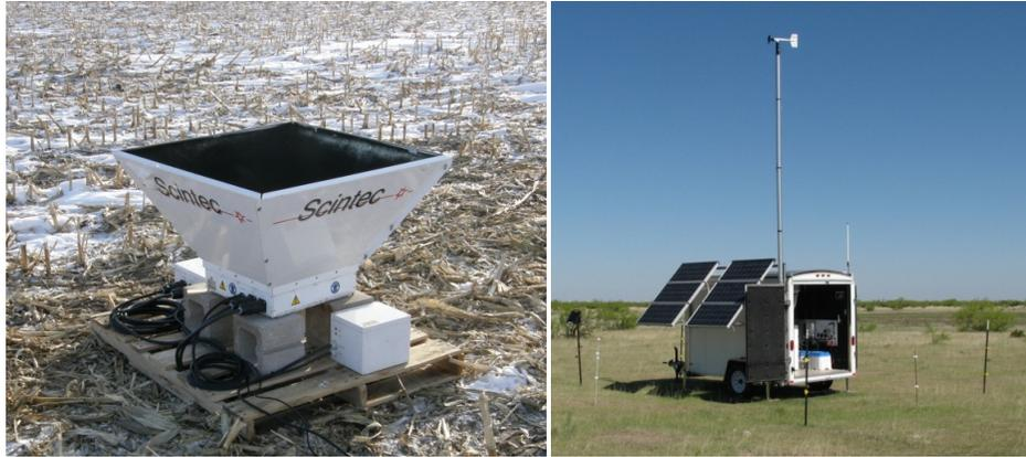
**Figure 8-2** *Left:* Scintec SFAS sodar unit. *Right:* Atmospheric Research & Technology VT-1 sodar unit enclosed within a trailer. (Source: AWS Truepower)
