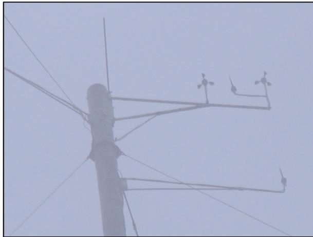
**Figure 7-5.** This sensor configuration is not recommended, as interference between sensors could produce inaccurate readings. (Source: AWS Truepower)
