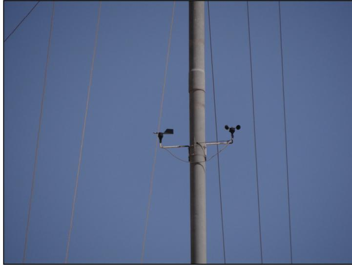
**Figure 7-4.** A poor sensor configuration. The anemometer booms are too short compared to the tower width, and likely would result in a large influence of the tower on the anemometer readings. (Source: AWS Truepower)
