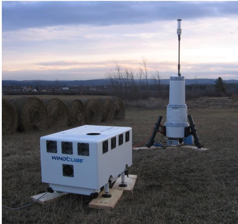
**Figure 8-3** Two commercial lidar units: a Leosphere Windcube V1 (left) and a 150-series ZephIR. (Source: AWS Truepower)
