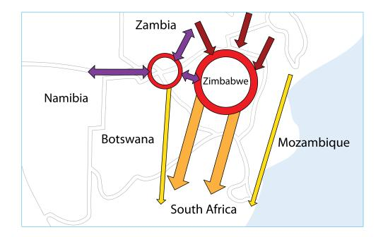
The arrows to the North of the ring are corridors that facilitate injection of generation from Malawi, Mozambique, Zambia and DRC. Projects are already proposed or in progress to upgrade the Kafue-Livingstone and North-West Botswana (Maun-Pandamatenga in figure 9) transmission lines. Two major power transfer routes into South Africa are provided from this central hub. The two routes would be designed to provide the redundancy required to improve reliability, stability and security.
