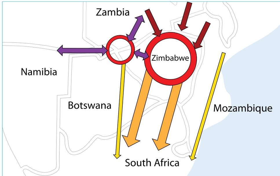
The arrows to the North of the ring are corridors that facilitate injection of generation from Malawi, Mozambique, Zambia and DRC. Projects are already proposed or in progress to upgrade the Kafue-Livingstone and North-West Botswana (Maun-Pandamatenga in figure 9) transmission lines. Two major power transfer routes into South Africa are provided from this central hub. The two routes would be designed to provide the redundancy required to improve reliability, stability and security.
