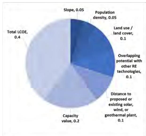
**FIGURE 11:** Example of zoning criteria weights used to calculate cumulative suitability score.
