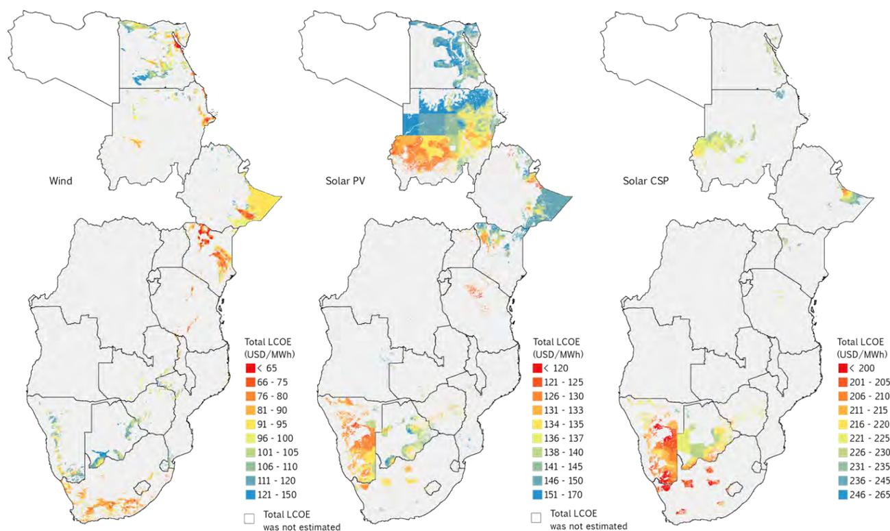
**FIGURE 1:** Average total levelized cost of electricity (LCOE) of wind (A), solar PV (B), and solar CSP (C) zones estimated using resource quality, distance to the nearest transmission line or substation, and distance to the nearest road.
