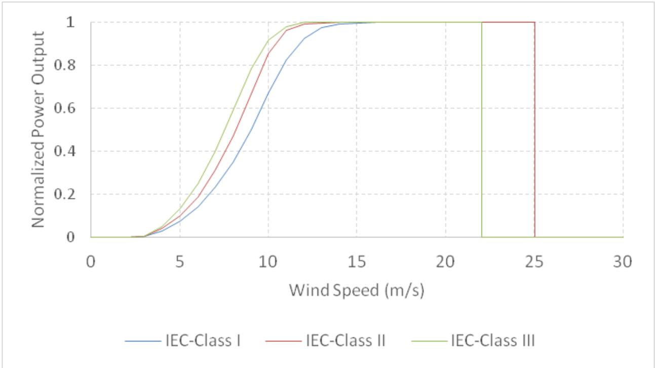
**FIGURE 6:** Normalized power curves for different IEC class turbines reproduced from [King et al., 2014].
