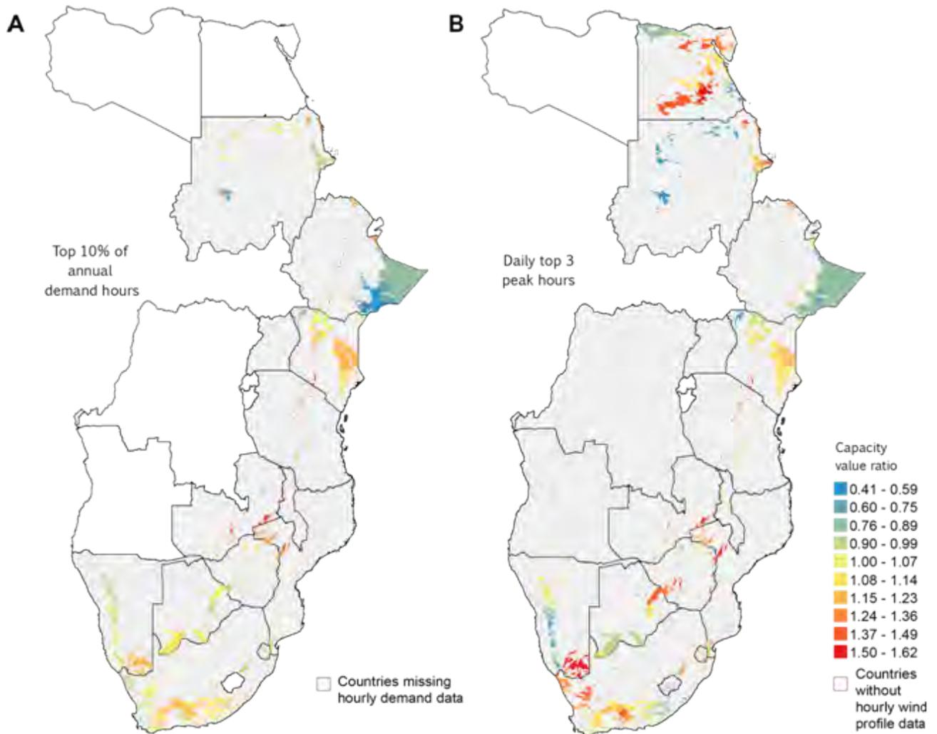
**FIGURE 23:** Comparison of capacity value ratios for ACEC wind zones.
