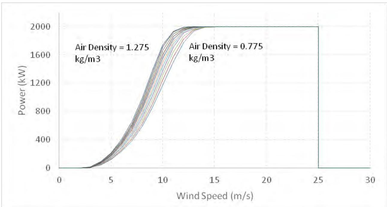
**FIGURE 7:** Adjusted IEC Class II power curves for air densities ranging from 1.275 kg/m<sup>3</sup> to 0.775 kg/m<sup>3</sup> (from left to right, respectively).
