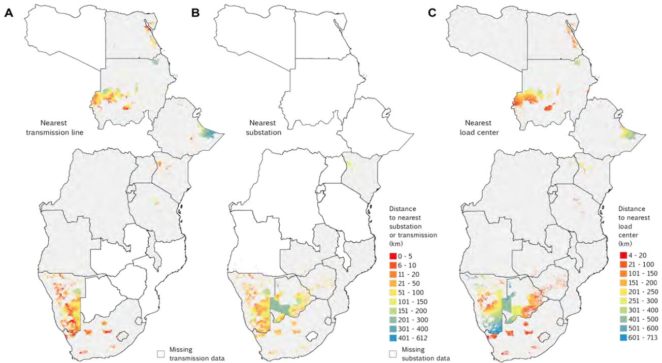
**FIGURE 31:** Comparison of distance to nearest transmission (A) and substation (B) with distance to nearest load center (C) for solar CSP zones.
