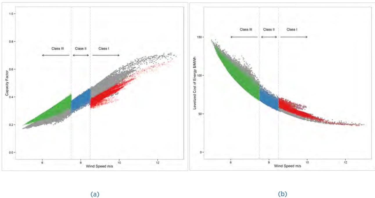
**FIGURE 8:** Relationship between average wind speed and estimated capacity factor (A) and levelized cost of energy (B) across the Africa Clean Energy Corridor.
