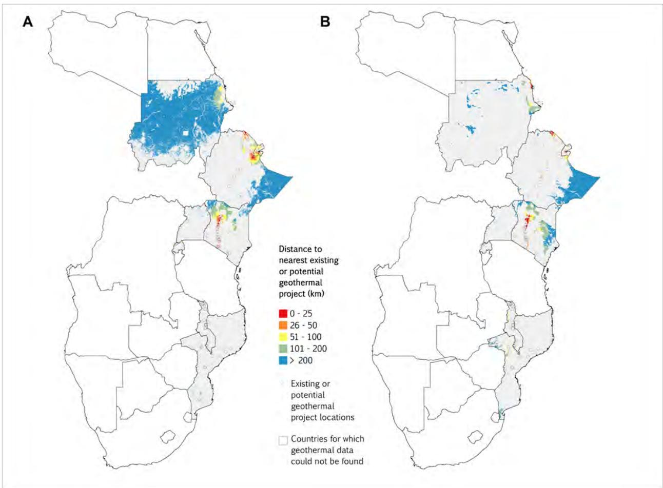
**FIGURE 33:** Distance to nearest existing or potential geothermal project for each solar PV (A) and wind (B) zone.
