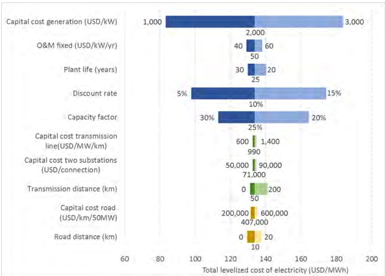
**FIGURE 39:** Total levelized cost of electricity (LCOE) sensitivity analysis for Solar PV.
