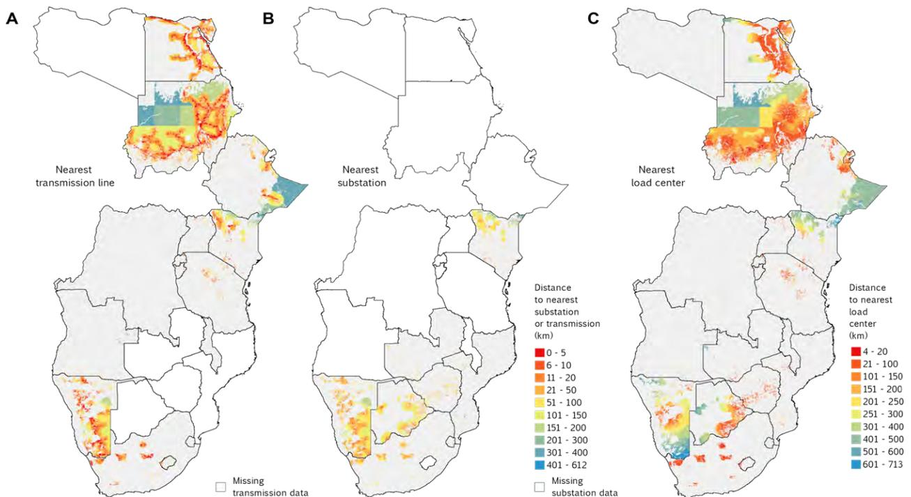
**FIGURE 30:** Comparison of distance to nearest transmission (A) and substation (B) with distance to nearest load center (C) for solar PV zones.
