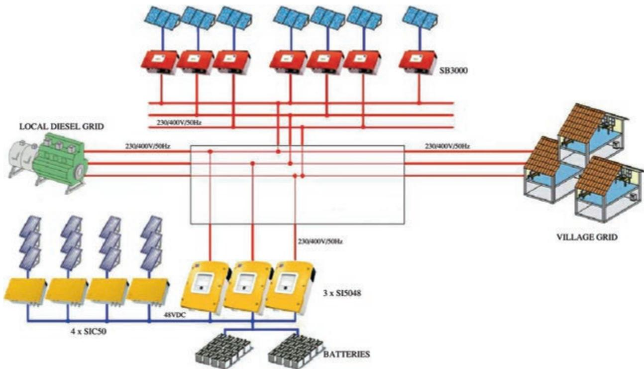
**Figure 4. Cluster block diagram for Tokelau solar project**
