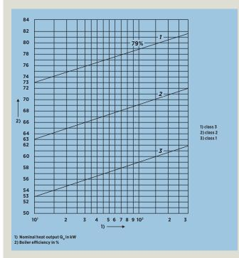
FIGURE 4: EXAMPLE FROM THE EN 303-5:1999 STANDARD FOR HEATING BOILERS ON THRESHOLD VALUES SETTING
