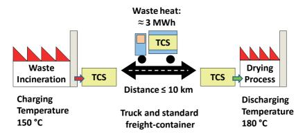
Figure 6 - Mobile Sorption Storage System for Industrial Waste Heat Utilisation
