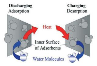
Figure 5 - TES De/Adsorption Process
