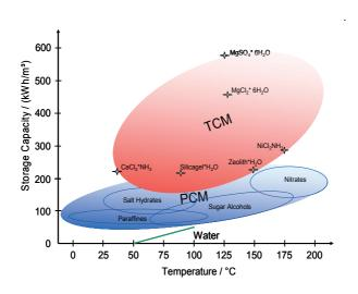
Figure 7 – Storage Capacity vs. Temperature for Sensible, Latent and Thermochemical TES [10]
