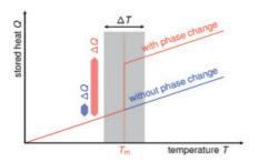
Figure 3 – Stored Heat vs. Temperature for Sensible (without phase change) and Latent TES [4]
