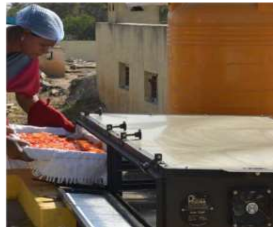
Solar Bubble Dryer
