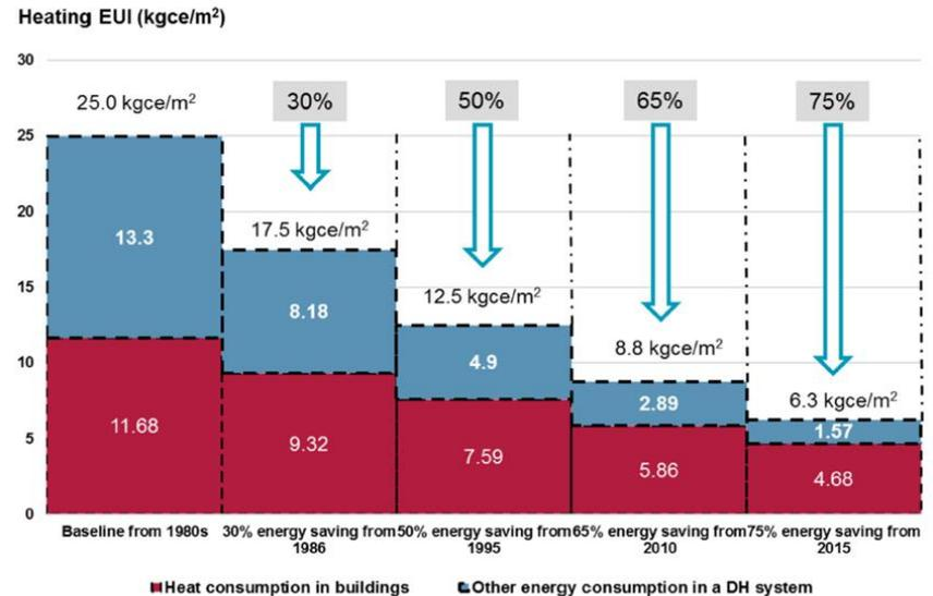
Fig. 4. Theoretical energy consumption of different percent of energy saving buildings in Beijing.
