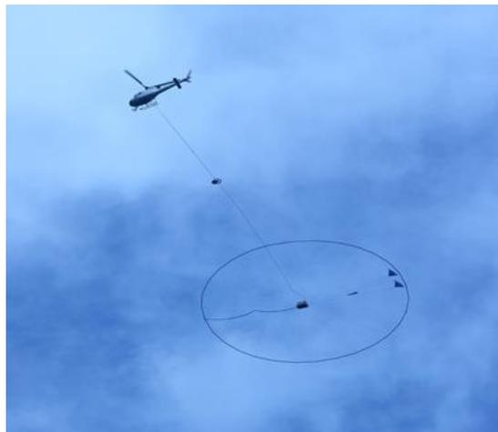
Air-borne Gravity Gradiometer (AGG)
