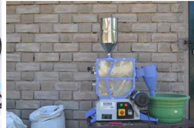
Efficient huller, polisher, de-stoner etc for remote tribal and rural areas- dependent on diesel
