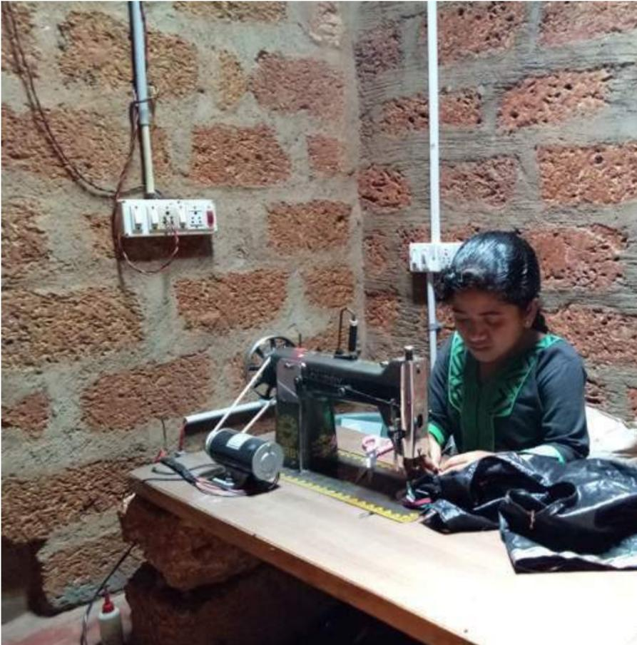
Sewing machine with efficient motor, belt and pedal; combined with appropriate financial models
