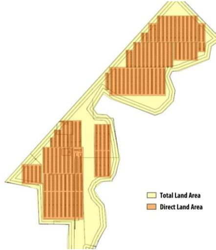
Typically 28-36 MW/km<sup>2</sup> Fixed-Tilt PV
