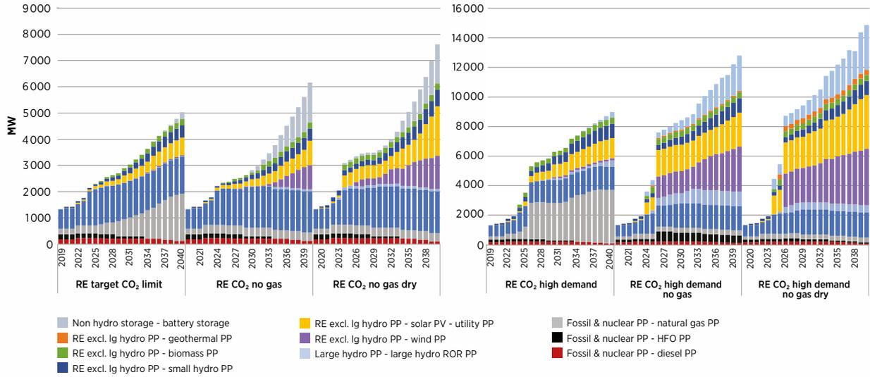
**Figure 3 Comparison of new generation capacity for the different scenarios**
