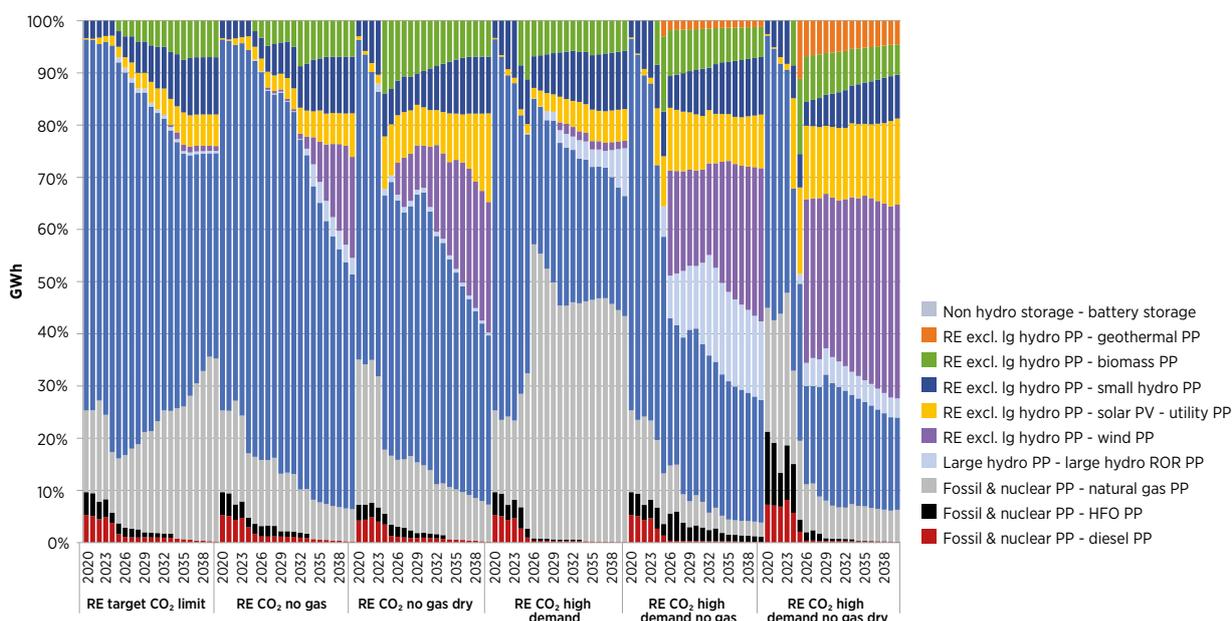
**Figure 2 Comparison of electricity generation capacity between different scenarios**
