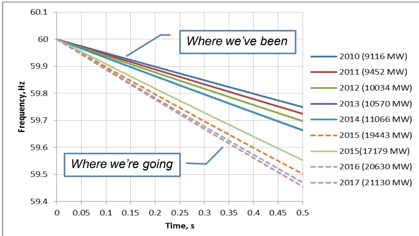
**Calculated ERCOT System Frequency after 2750 MW Generation Trip
