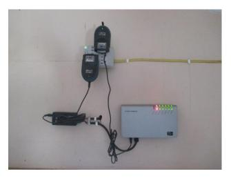
Data logger and associated power supplies (located indoors)
