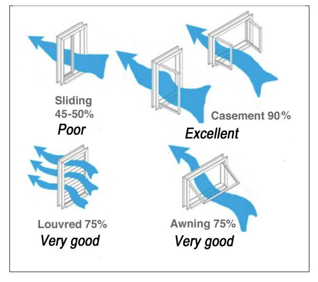
Figure 7. Ventilation through different types of windows
