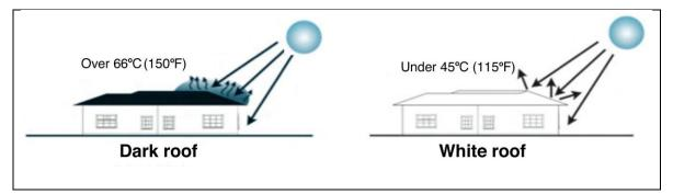
A few houses have flat concrete roofs that must be coated with a waterproofing product. White or a metallic reflective colour is preferable to darker colours for this product.
