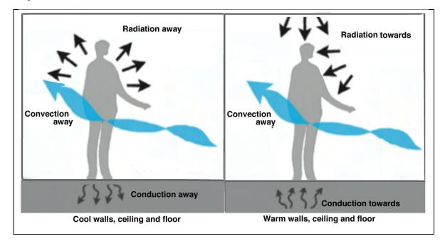
Figure 1. Heat transfer and human comfort at a constant air flow
