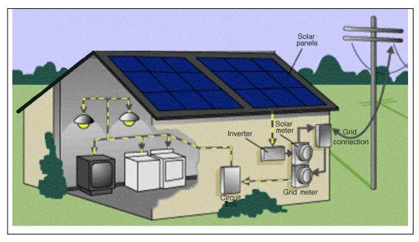
Figure 9. Grid-connected solar installation components
