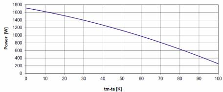
Power output per collector unit at specific values of  $t_m$ - $t_a$  and G:
