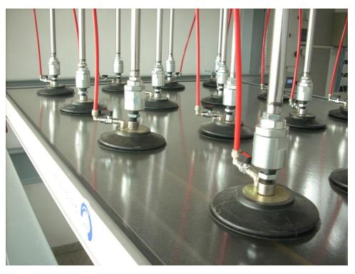
Positive pressure applied on the cover of the collector by using suction cups.
