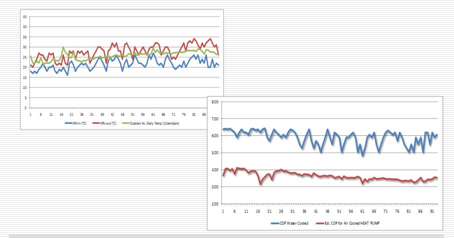
Inlet and outlet temperatures of the water from the VRV and daily average outside air temperature for the period from 01/07/2010 to 31/08/2010
