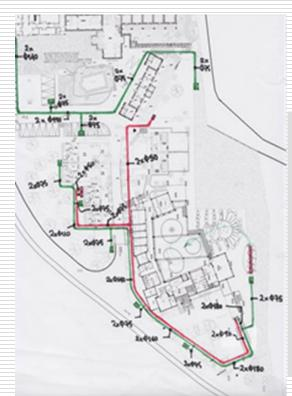
The application of the system was implemented using Vertical Earth (Geothermal) Heat Exchangers (VEHE) which settled in the surroundings of the buildings. The energy is pumped or rejected into the subsurface and is driven through central piping to individual plant rooms where the thermal gradient is changed through water-cooled VRV heat pumps and finally is circulated for indoor usage.
