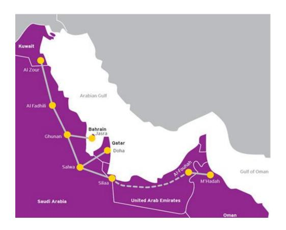
A 400kV 'backbone' electrical transmission link between all GCC Member States
