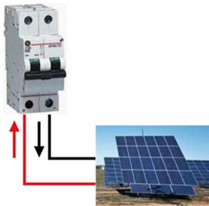
Preferred connection of array to a Polarised Double Pole DC Circuit Breaker with markings on bottom of CB
