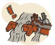
The intake has suffered structural damage, causing no water diversion or loss of flow in a MHP system.
