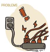
Too many appliances or devices are connected to a single electrical circuit, drawing more current than it can safely handle.
