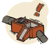
The forebay is obstructed by an excessive accumulation of debris, such as leaves, sediment, sticks, and other waste. This blockage prevents the free flow of water into the penstock and turbine.
