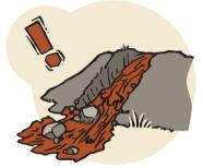
A slope failure occurring in the upper part of a river or watershed, which can increased turbidity and damage to downstream ecosystems and infrastructure.
