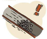
There is a physical obstruction inside the penstock or any other water channel (like the headrace channel) that restricts the flow of water.
