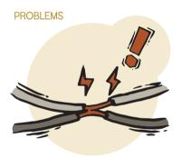
A faulty connection in an electrical circuit that allows current to travel along an unintended, low-resistance path, causing a sudden and very large surge of electric current.
