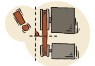
The belt's path is not in proper alignment with the pulleys it drives, leading to uneven wear, noise, and reduced performance.
