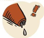
The opening through which a jet of water is directed onto the turbine is partially or completely blocked.
