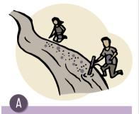
The flow rate is determined by measuring the speed and concentration of the cloud of salt using a sensor as it passes downstream.
