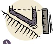
Using a hose or tube filled with water to measure the difference in elevation (head) between two points
