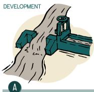
The intake is the entry point where water is diverted from a river or stream into the MHP system.
