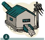
The building at the end of a micro-hydropower system that houses the turbine, generator, and Electronic Load Controller (ELC).
