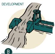
A weir is a low dam built across the water source to raise the water level to ensure a consistent flow of water into the intake.
