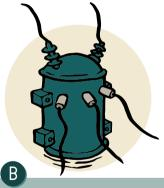
Transformer can either step up the voltage for efficient long-distance transmission or step down the voltage for safe use by consumers.
