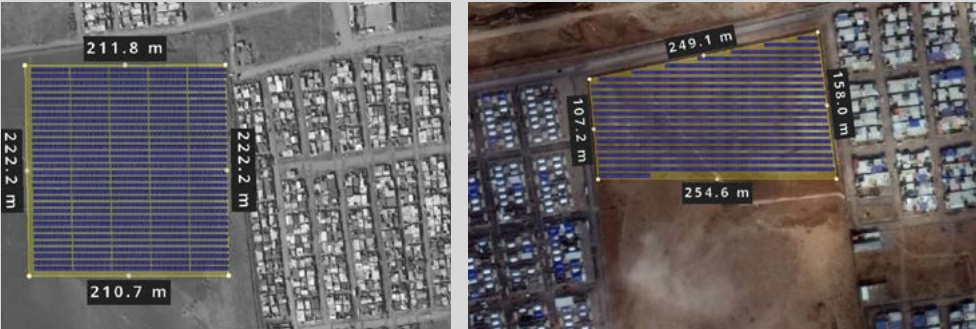
FIGURE 4.9 Proposed 6.6 MW solar PV installation in Domiz 1 (left) and 2.5 MW solar PV installation in Domiz 2 (right)
