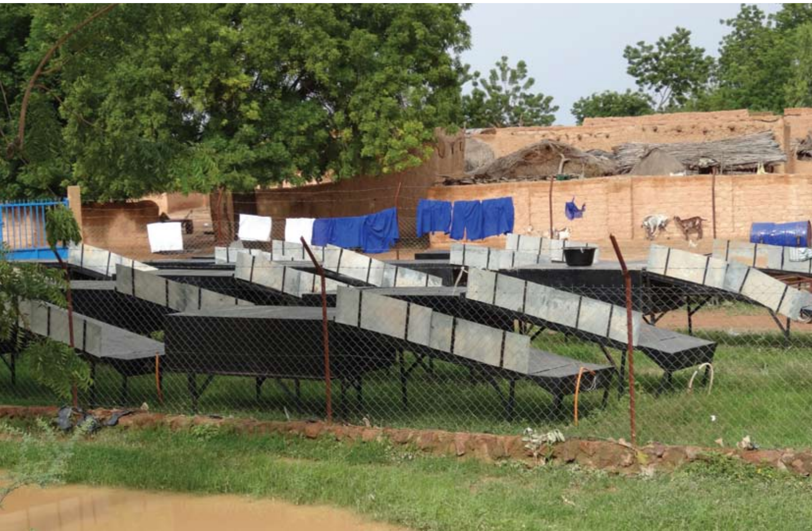
Solar dryers in Makalondi village Photo: IRENA/H. Lucas
