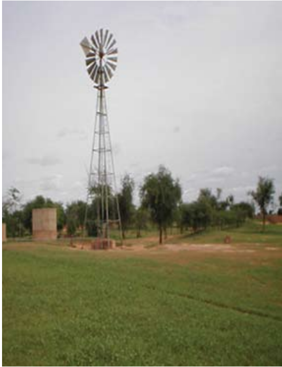
Wind water pumping system in Chikal village Courtesy: Ministry of Energy and Petroleum, Niger
