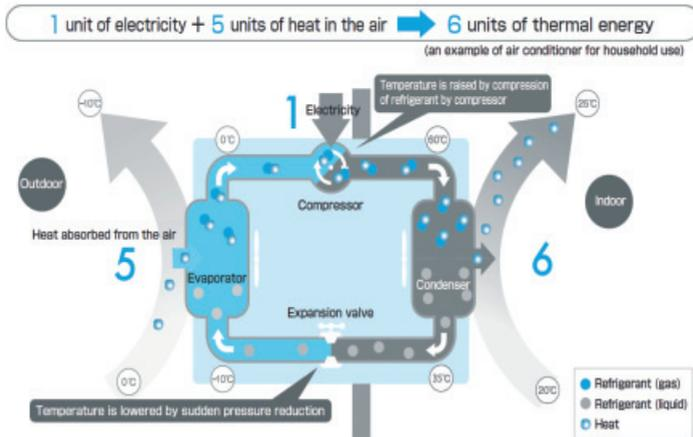
Figure 2 – Mechanism of Heat Pump [1]
